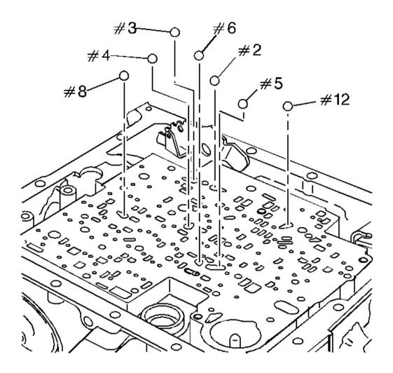
Fig. 49: Identifying Valve Body Checkballs Courtesy of GENERAL MOTORS CORP.
