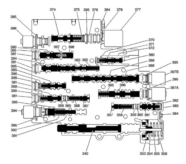
Fig. 18: Valve Trains Component Location Courtesy of GENERAL MOTORS CORP.
