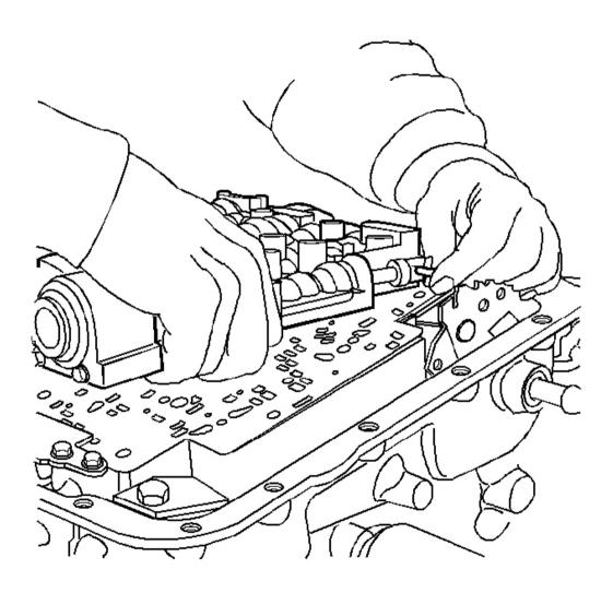
Fig. 285: Installing Valve Body Courtesy of GENERAL MOTORS CORP.
