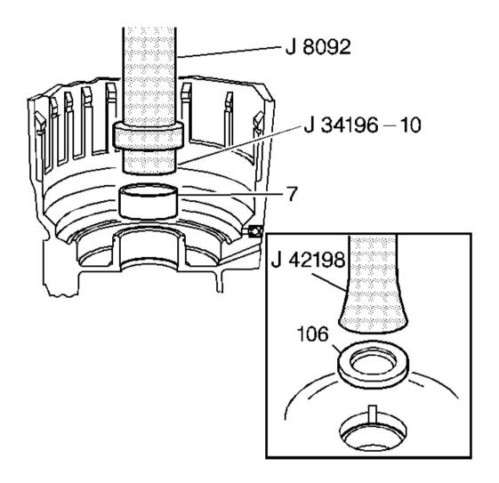
Fig. 98: View Of Case Bushing & Case Rear Oil Seal Courtesy of GENERAL MOTORS CORP.
