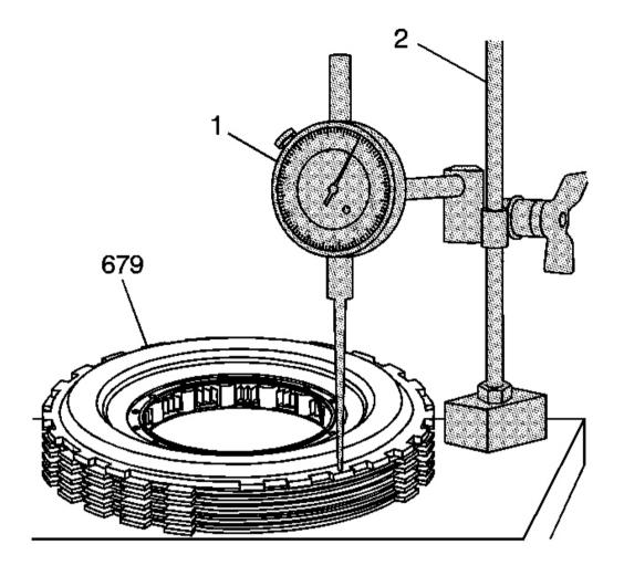
Fig. 113: Measuring Clutch Pack Height With J 8001 Courtesy of GENERAL MOTORS CORP.
