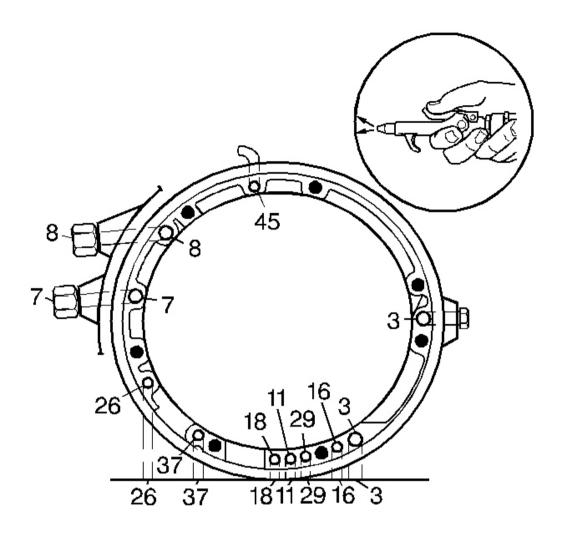
Fig. 86: Identifying Case Fluid Passages Courtesy of GENERAL MOTORS CORP.
