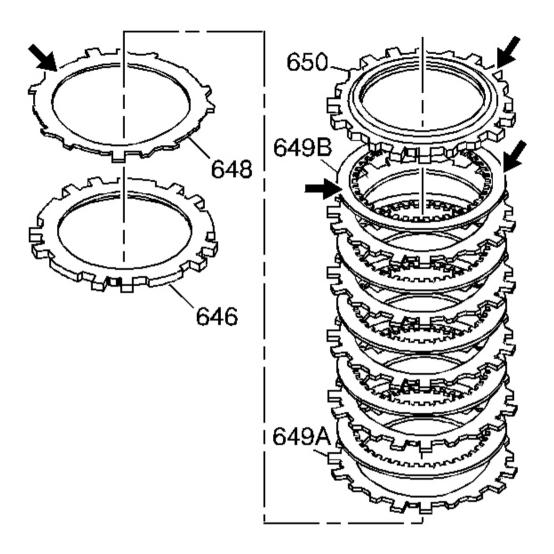
Fig. 176: Inspecting Forward Clutch Assembly For Wear Or Damage Courtesy of GENERAL MOTORS CORP.
