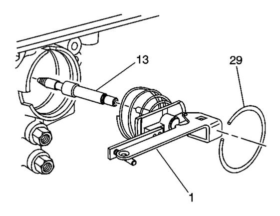
Fig. 31: Locating Servo Cover Retaining Ring Courtesy of GENERAL MOTORS CORP.
