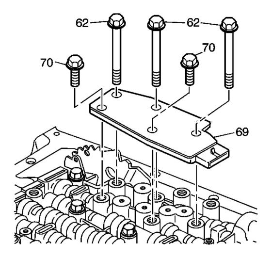
Fig. 288: TFP Manual Valve Position Switch Retaining Bolts Courtesy of GENERAL MOTORS CORP.
