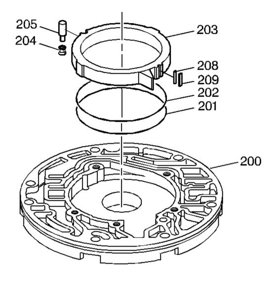
Fig. 210: Identifying Pump Slide Components Courtesy of GENERAL MOTORS CORP.
