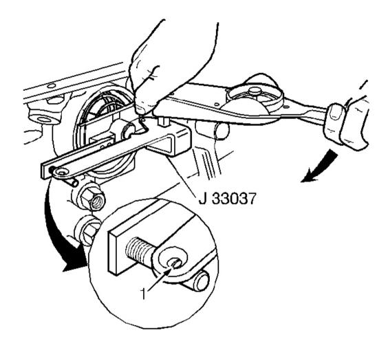
Fig. 302: Identifying Gage Slot Courtesy of GENERAL MOTORS CORP.
