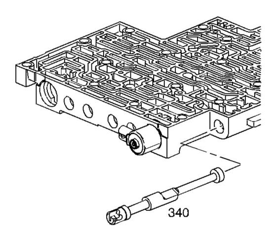
Fig. 271: View Of Manual Valve Courtesy of GENERAL MOTORS CORP.
