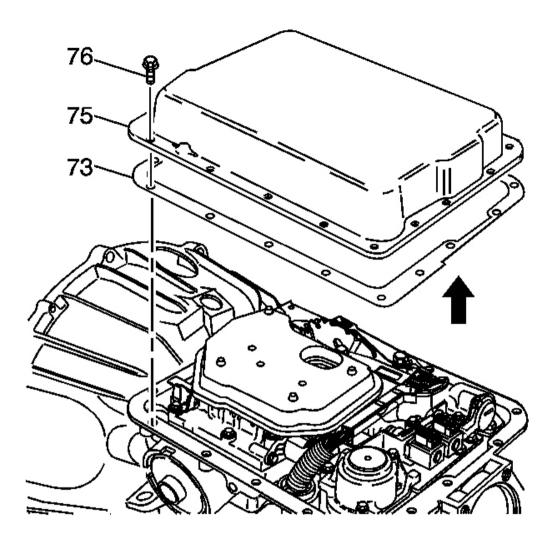
Fig. 36: View Of Transmission Oil Pan & Gasket Courtesy of GENERAL MOTORS CORP.
