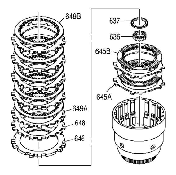
Fig. 148: View Of Forward Clutch Plates Courtesy of GENERAL MOTORS CORP.
