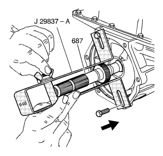
Fig. 35: Installing J 29837-A Courtesy of GENERAL MOTORS CORP.
