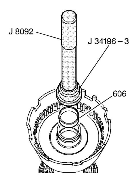
Fig. 194: Installing Reverse Input Clutch Rear Bushing Courtesy of GENERAL MOTORS CORP.
