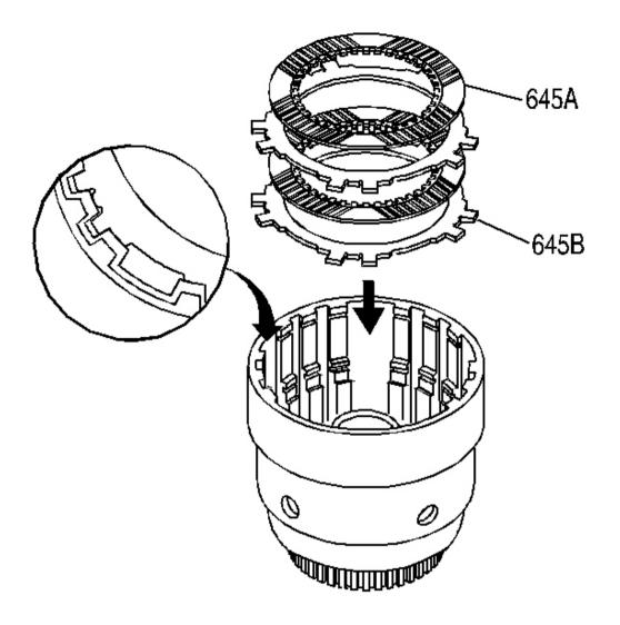
Fig. 167: Aligning Overrun Clutch Plates Courtesy of GENERAL MOTORS CORP.
