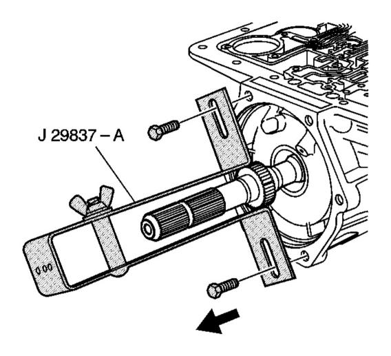
Fig. 72: Identifying J 29837-A Courtesy of GENERAL MOTORS CORP.
