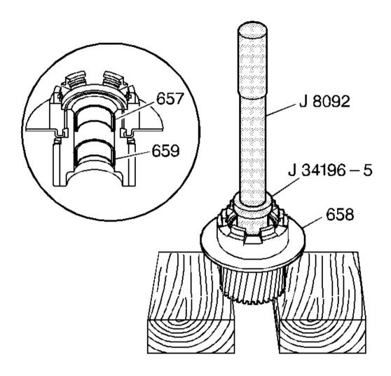
Fig. 139: Removing Input Sun Gear Front Bushing Courtesy of GENERAL MOTORS CORP.
