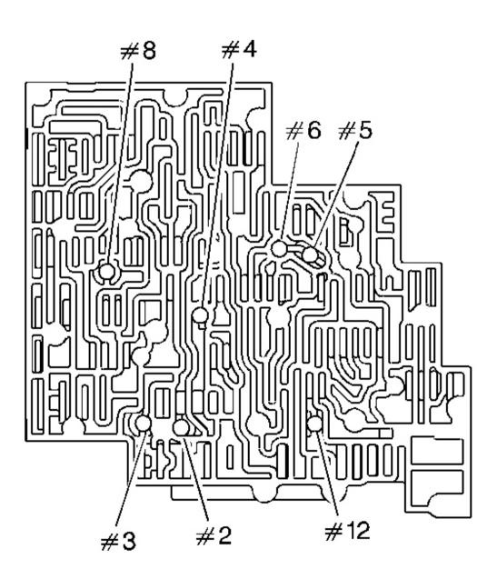
Fig. 284: Identifying Checkball Installation Positions Courtesy of GENERAL MOTORS CORP.
