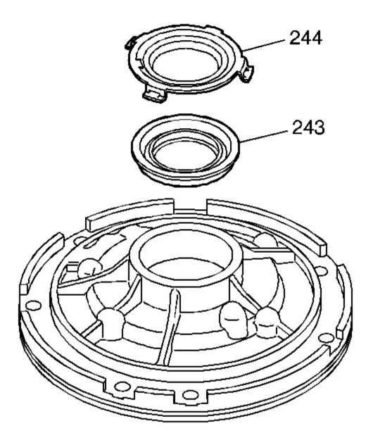
Fig. 213: Locating Front Helix Retainer & Oil Seal Assembly Courtesy of GENERAL MOTORS CORP.
