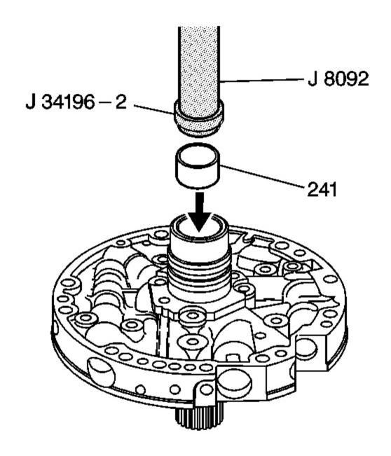
Fig. 231: Installing Stator Shaft Rear Bushing Courtesy of GENERAL MOTORS CORP.
