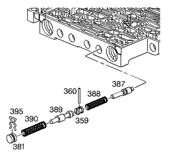
Fig. 264: View Of Reverse Abuse Valve & 3-2 Downshift Valve Courtesy of GENERAL MOTORS CORP.
