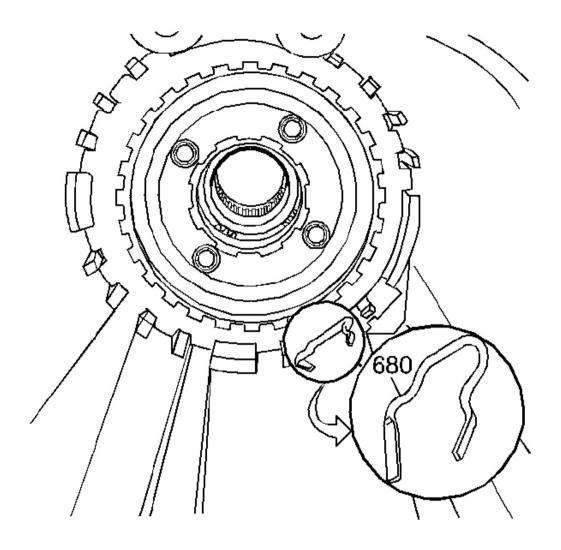
Fig. 119: View Of Low And Reverse Clutch Support Retainer Spring Courtesy of GENERAL MOTORS CORP.
