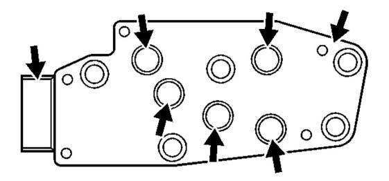
Fig. 287: Inspection Areas On Transmission Fluid Pressure (TFP) Manual Valve Position Switch Assembly Courtesy of GENERAL MOTORS CORP.
