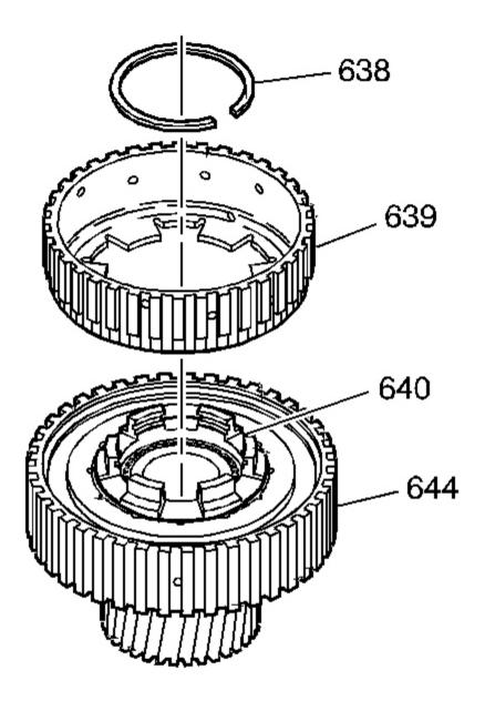
Fig. 169: Locating Overrun Clutch Courtesy of GENERAL MOTORS CORP.
