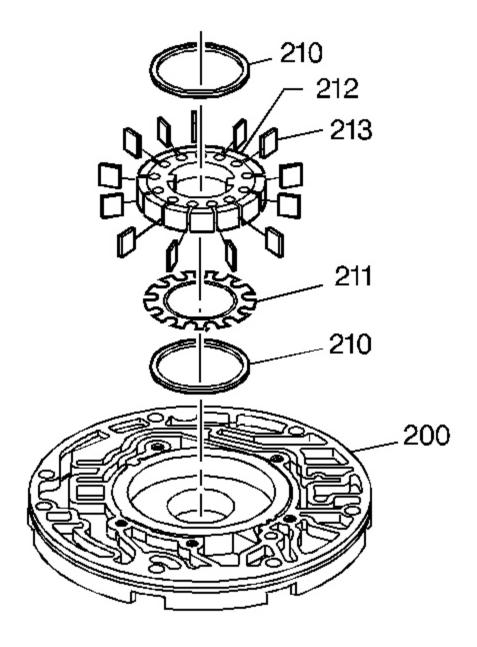
Fig. 209: Identifying Pump Vane Ring Assemblies Courtesy of GENERAL MOTORS CORP.
