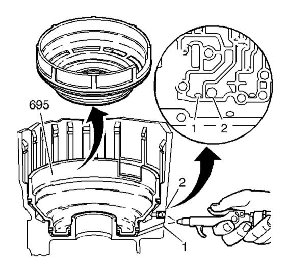
Fig. 84: Blowing Air Into Case Passage Courtesy of GENERAL MOTORS CORP.
