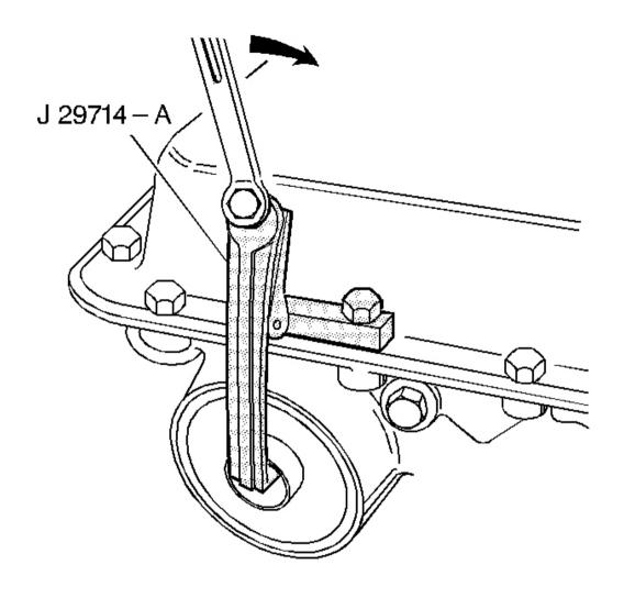
Fig. 27: Compressing Servo Cover With J 29714-A Courtesy of GENERAL MOTORS CORP.
