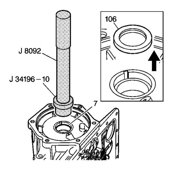
Fig. 97: Identifying Case Rear Oil Seal & Case Bushing Courtesy of GENERAL MOTORS CORP.
