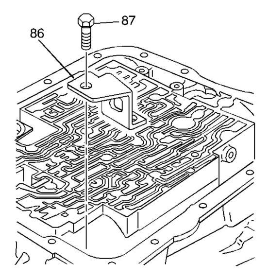
Fig. 81: View Of Parking Lock Bracket & Bolt Courtesy of GENERAL MOTORS CORP.
