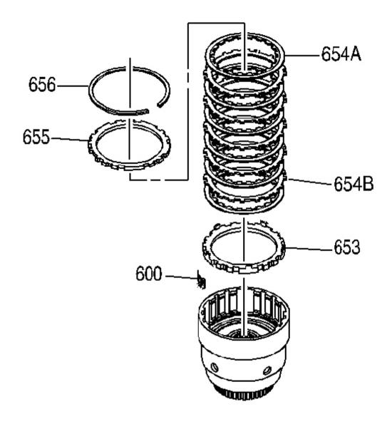
Fig. 146: Locating 3rd & 4th Clutch Backing Plate Retainer Ring Courtesy of GENERAL MOTORS CORP.
