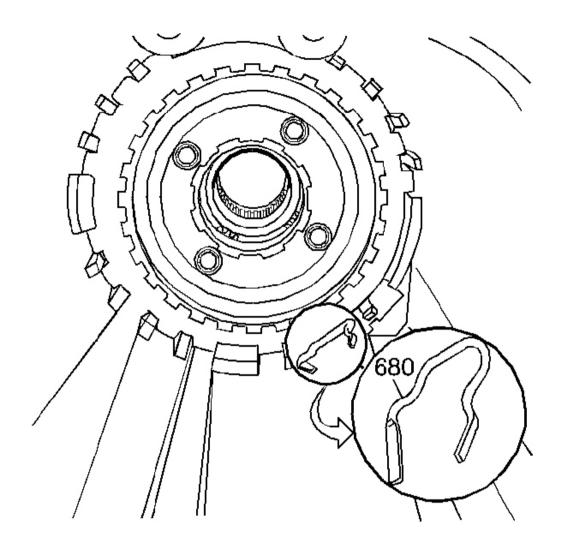
Fig. 75: View Of Low And Reverse Clutch Support Retainer Spring Courtesy of GENERAL MOTORS CORP.
