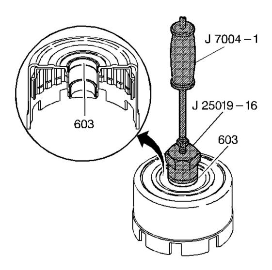
Fig. 191: Identifying Reverse Input Clutch Front Bushing Courtesy of GENERAL MOTORS CORP.
