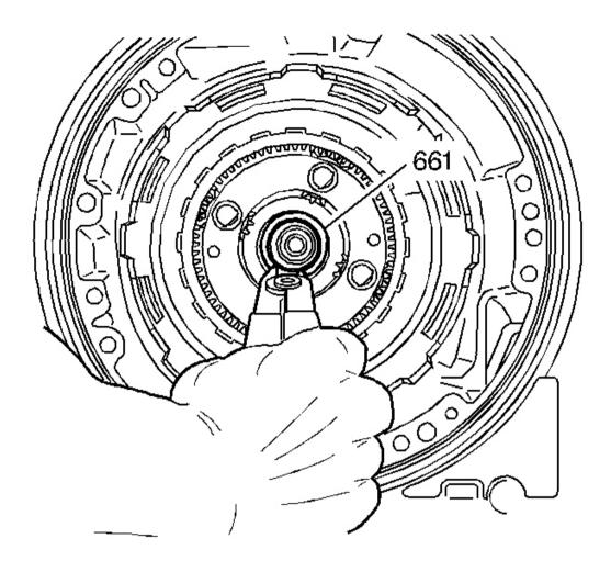
Fig. 143: View Of Output Shaft To Input Carrier Retainer Courtesy of GENERAL MOTORS CORP.
