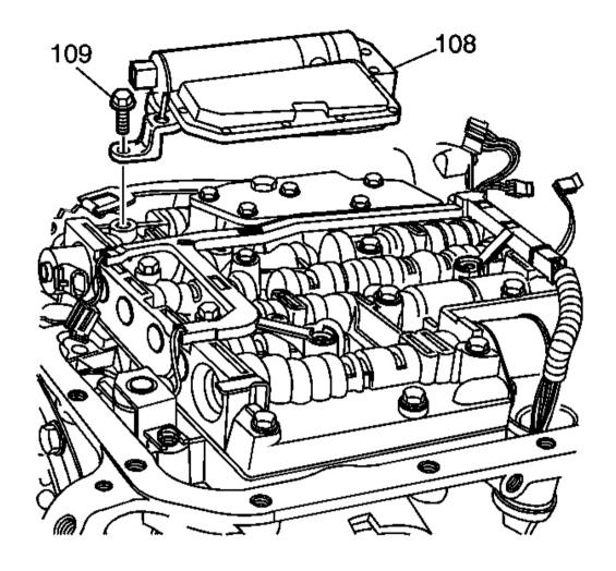
Fig. 40: Identifying Secondary Fluid Pump Courtesy of GENERAL MOTORS CORP.
