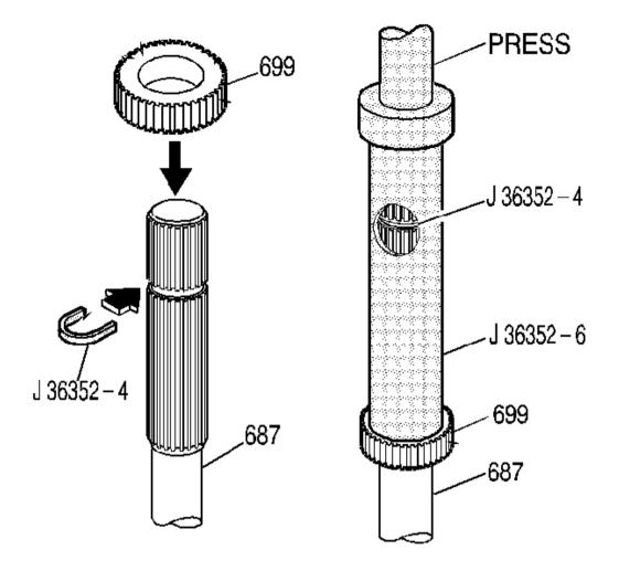
Fig. 135: Pressing Internal Speed Sensor Rotor Onto Output Shaft Courtesy of GENERAL MOTORS CORP.
