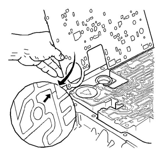
Fig. 85: Inspecting Spacer Plate To Case Gasket For Witness Marks Courtesy of GENERAL MOTORS CORP.
