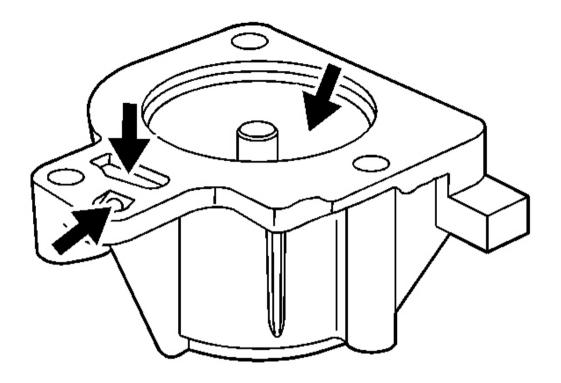
Fig. 276: Locating 1-2 Accumulator Housing Inspection Areas Courtesy of GENERAL MOTORS CORP.
