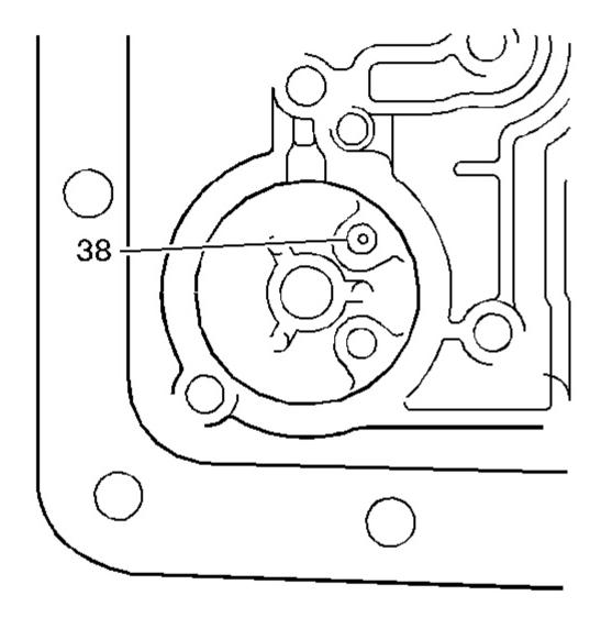
Fig. 88: Locating Orifice Cup Plug Courtesy of GENERAL MOTORS CORP.
