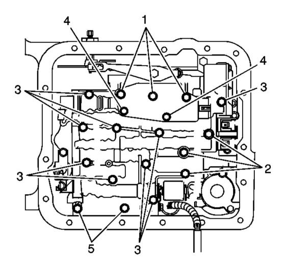
Fig. 290: Locating Valve Body Bolts Courtesy of GENERAL MOTORS CORP.
