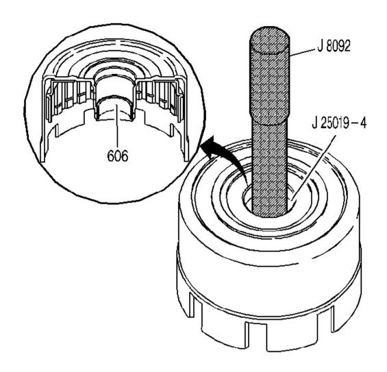
Fig. 192: Locating Reverse Input Clutch Rear Bushing Courtesy of GENERAL MOTORS CORP.
