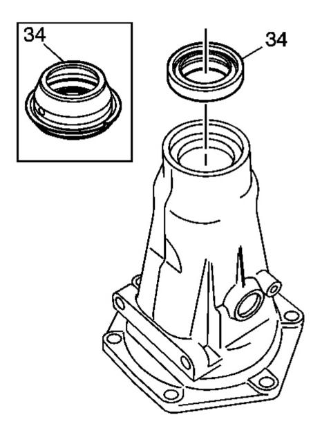
Fig. 311: View Of Case Extension Oil Seal Assembly Courtesy of GENERAL MOTORS CORP.
