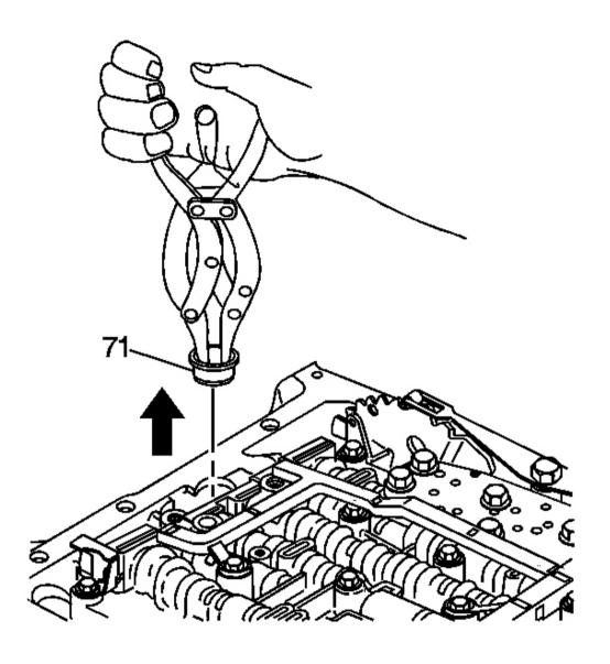
Fig. 38: Removing Oil Filter Seal Courtesy of GENERAL MOTORS CORP.
