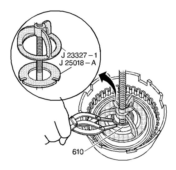
Fig. 198: View Of Reverse Input Clutch Spring Retainer Ring Courtesy of GENERAL MOTORS CORP.
