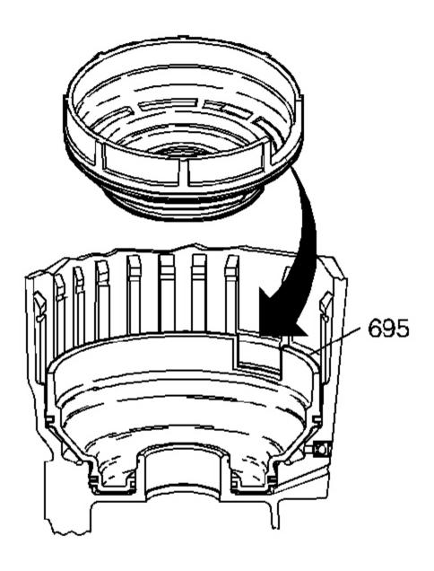
Fig. 101: Aligning Parking Brake Pawl Window With Notch In Piston Courtesy of GENERAL MOTORS CORP.
