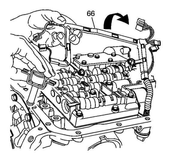
Fig. 44: Removing TCC Solenoid And Wiring Harness Courtesy of GENERAL MOTORS CORP.
