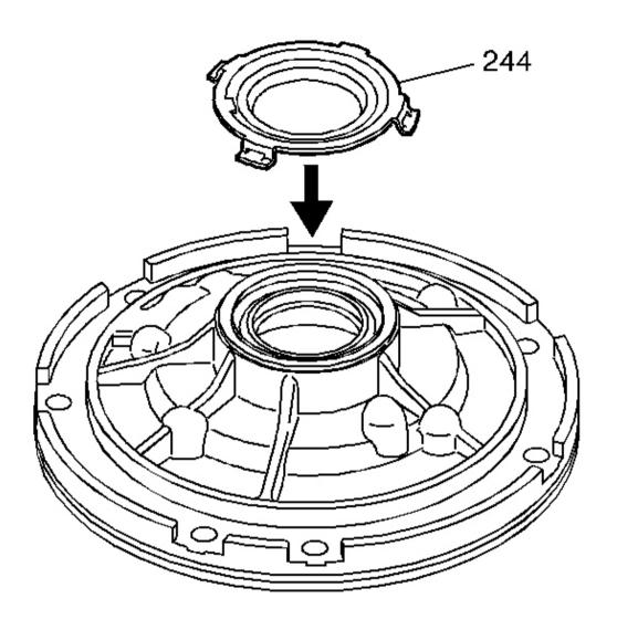
Fig. 218: Installing Front Helix Retainer Courtesy of GENERAL MOTORS CORP.
