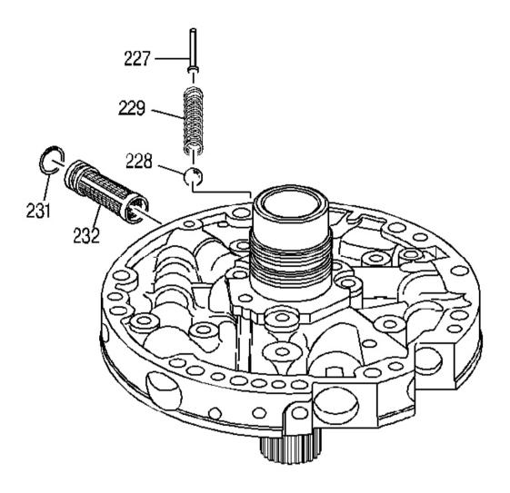
Fig. 224: Removing Oil Pump Cover Screen & Pressure Relief Components Courtesy of GENERAL MOTORS CORP.
