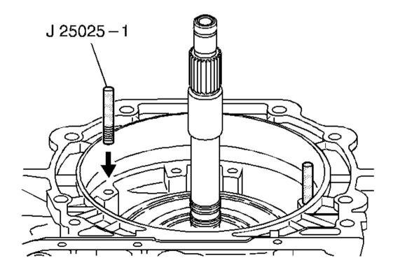
Fig. 237: Installing J 25025-1 Courtesy of GENERAL MOTORS CORP.
