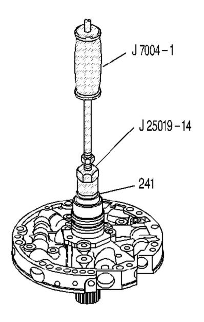
Fig. 229: Removing Stator Shaft Rear Bushing Courtesy of GENERAL MOTORS CORP.
