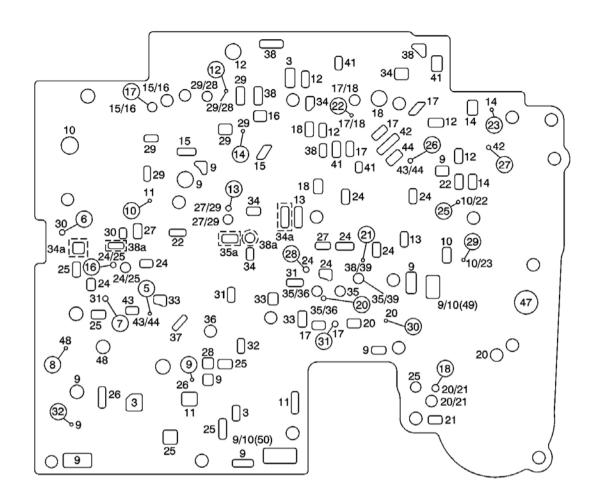
Fig. 341: Spacer Plate Fluid Passages Courtesy of GENERAL MOTORS CORP.
