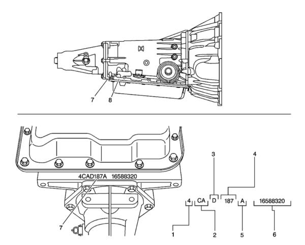
Fig. 322: Transmission ID Information Courtesy of GENERAL MOTORS CORP.
