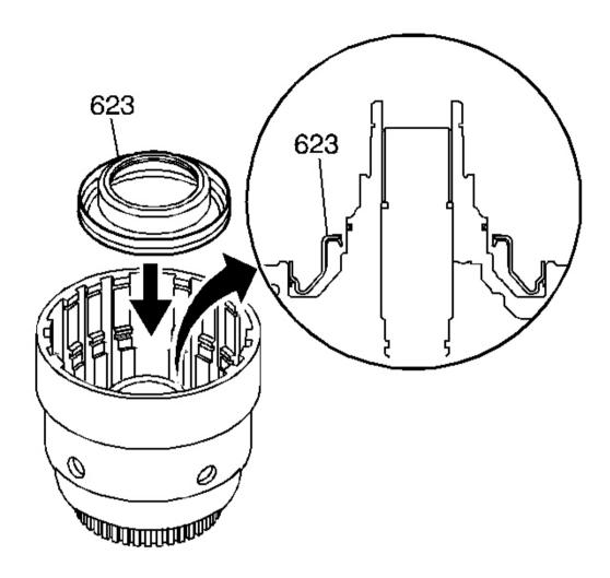
Fig. 154: Identifying 3rd & 4th Clutch Piston Inspection Areas Courtesy of GENERAL MOTORS CORP.
