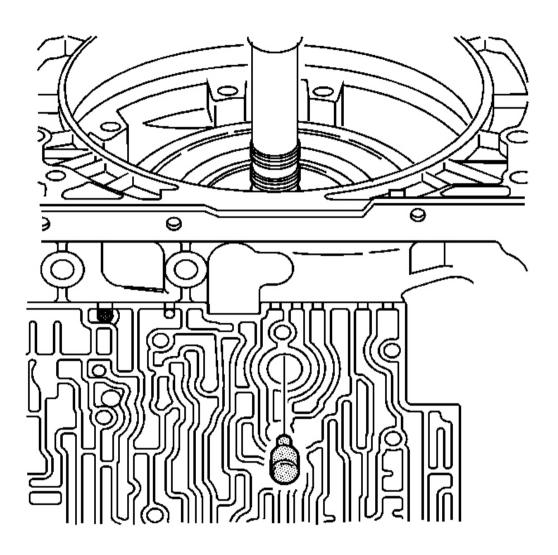
Fig. 63: Identifying Band Anchor Pin Courtesy of GENERAL MOTORS CORP.
