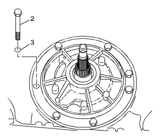
Fig. 242: Locating Pump To Case Bolts & O-Ring Seals Courtesy of GENERAL MOTORS CORP.
