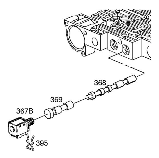
Fig. 252: Identifying 2-3 Shuttle Valve & Solenoid Components Courtesy of GENERAL MOTORS CORP.
