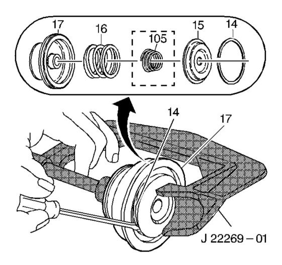
Fig. 304: Locating Servo Cushion Outer & Inner Spring With Retainer Courtesy of GENERAL MOTORS CORP.
