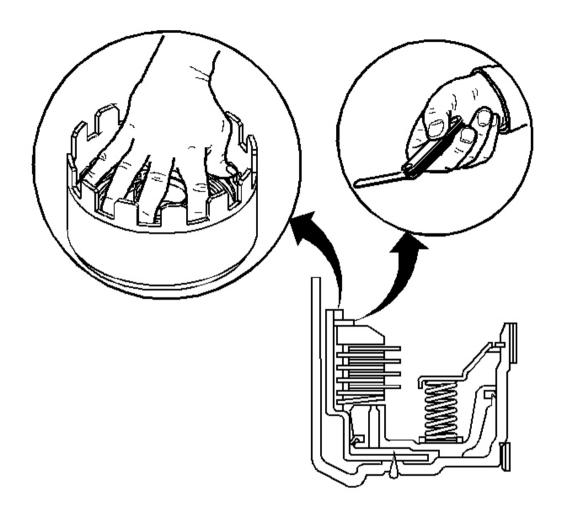
Fig. 201: Checking Reverse Input Clutch Plate Travel Courtesy of GENERAL MOTORS CORP.
