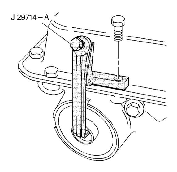
Fig. 307: Installing J 29714-A
