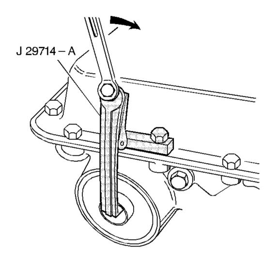
Fig. 308: Compressing Servo Cover With J 29714-A Courtesy of GENERAL MOTORS CORP.
