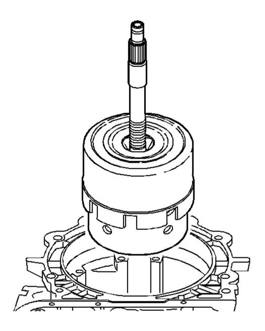
Fig. 64: Removing Input Housing And Shaft Assembly & Reverse Input Clutch Housing And Drum <u>Assembly</u> Courtesy of GENERAL MOTORS CORP.
