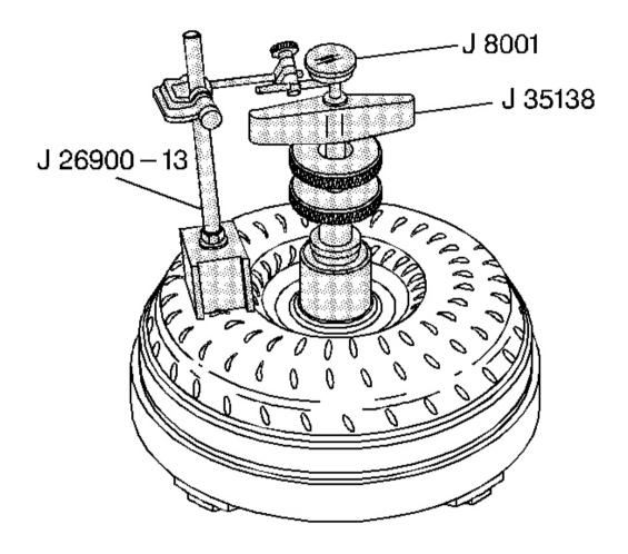
Fig. 319: Identifying J 35138, J 26900-13 & J 8001 Courtesy of GENERAL MOTORS CORP.
