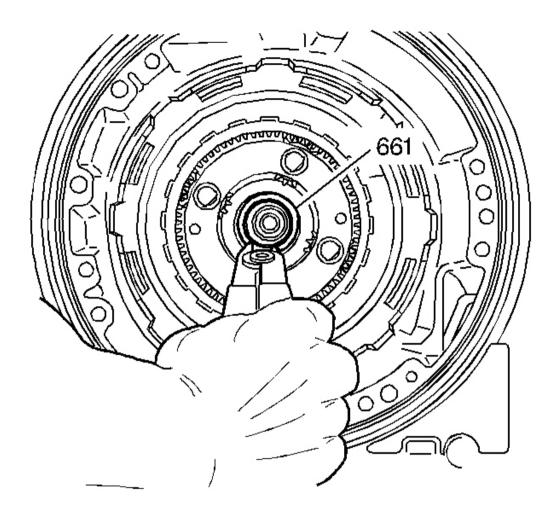
Fig. 66: View Of Output Shaft To Input Carrier Retainer Courtesy of GENERAL MOTORS CORP.
