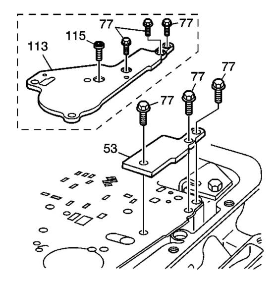
Fig. 281: View Of Spacer Plate Support Plate & Bolts Courtesy of GENERAL MOTORS CORP.
