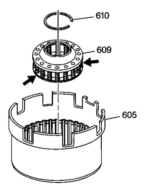
Fig. 197: Identifying Reverse Input Clutch Spring Assembly Courtesy of GENERAL MOTORS CORP.
