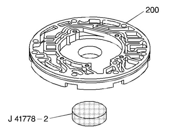
Fig. 216: Identifying J 41778-2 Courtesy of GENERAL MOTORS CORP.
