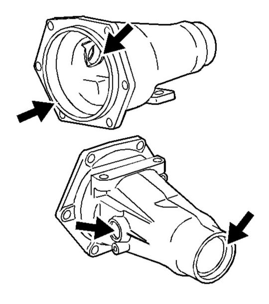
Fig. 310: Identifying Inspection Areas On Case Extension Courtesy of GENERAL MOTORS CORP.
