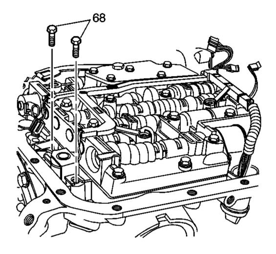
Fig. 289: Identifying TCC Solenoid Valve Mounting Bolts Courtesy of GENERAL MOTORS CORP.
