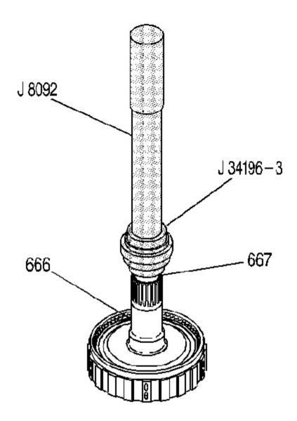
Fig. 131: View Of Reaction Carrier Shaft Rear Bushing Courtesy of GENERAL MOTORS CORP.
