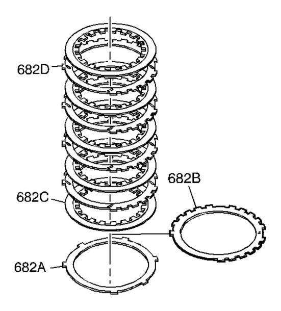
Fig. 114: View Of Clutch Pack Courtesy of GENERAL MOTORS CORP.
