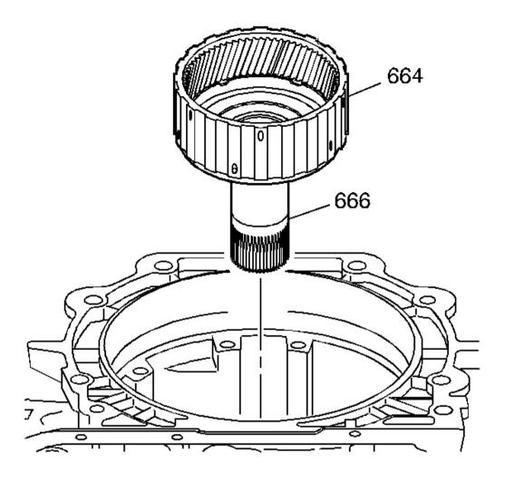
Fig. 68: Reaction Carrier Shaft Assembly & Input Internal Gear Courtesy of GENERAL MOTORS CORP.
