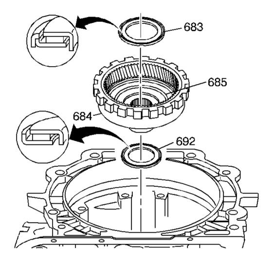
Fig. 78: View Of Reaction Carrier/Support Thrust Bearing Assembly Courtesy of GENERAL MOTORS CORP.
