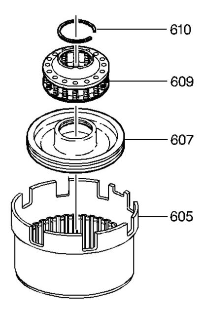
Fig. 189: Identifying Reverse Input Clutch Spring & Piston Assemblies Courtesy of GENERAL MOTORS CORP.
