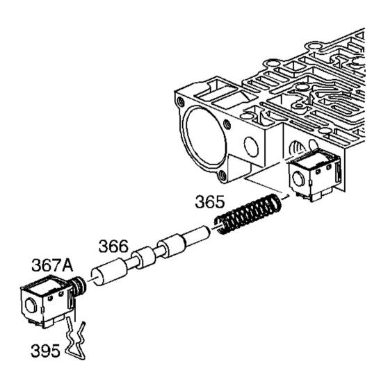
Fig. 269: Locating 1-2 Shift Valve & Solenoid Components Courtesy of GENERAL MOTORS CORP.
