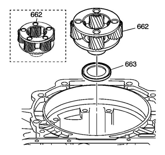
Fig. 67: Identifying Input Carrier Assembly Courtesy of GENERAL MOTORS CORP.
