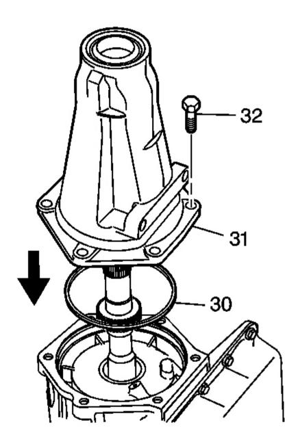
Fig. 315: Locating Case Extension Case Seal Courtesy of GENERAL MOTORS CORP.
