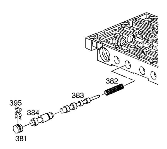
Fig. 262: View Of 4-3 Sequence Valve & 3-4 Relay Valve Courtesy of GENERAL MOTORS CORP.
