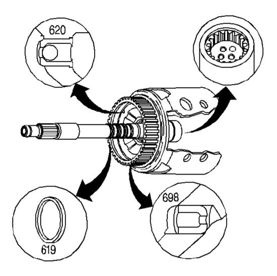
Fig. 151: Expanded View Of Input Housing Courtesy of GENERAL MOTORS CORP.
