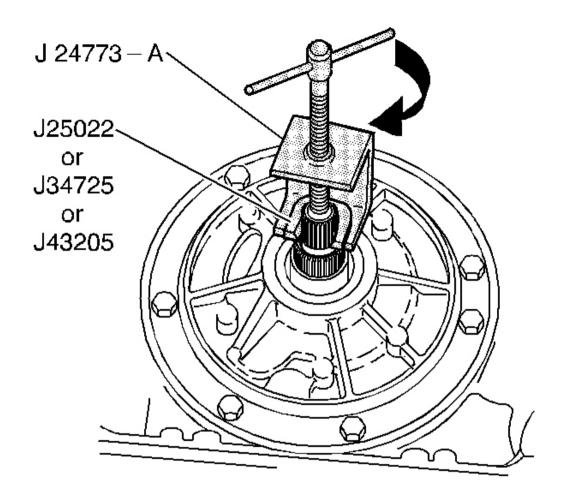
Fig. 57: Identifying J 24773-A Courtesy of GENERAL MOTORS CORP.
