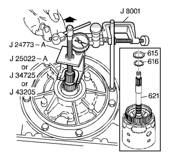
Fig. 59: Checking End Play With J 8001 Courtesy of GENERAL MOTORS CORP.
