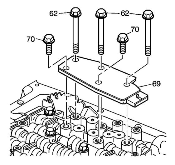
Fig. 45: TFP Manual Valve Position Switch Retaining Bolts Courtesy of GENERAL MOTORS CORP.
