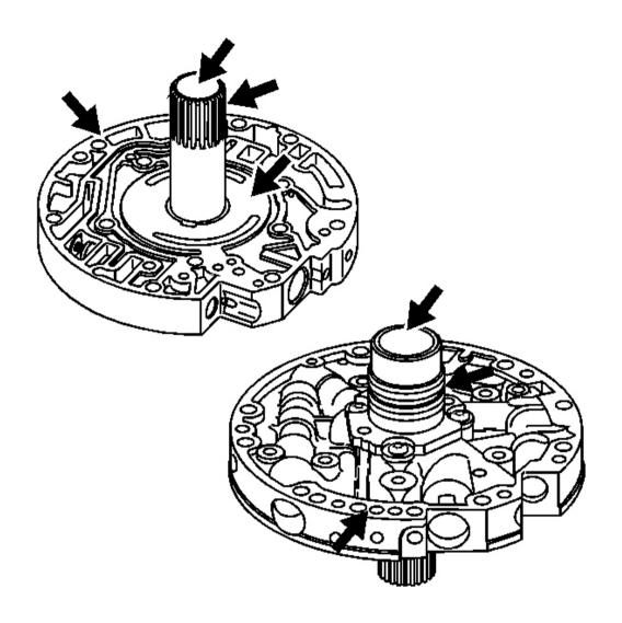
Fig. 227: View Of Pump Cover Inspection Areas Courtesy of GENERAL MOTORS CORP.
