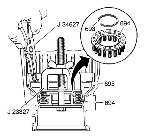
Fig. 102: View Of Low And Reverse Clutch Spring Assembly & Retainer Ring Courtesy of GENERAL MOTORS CORP.
