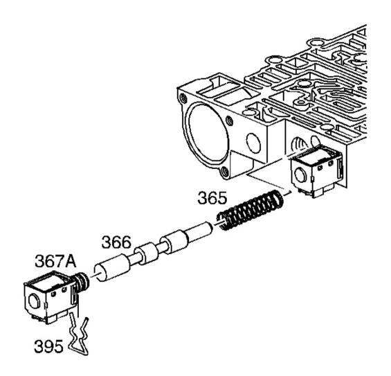
Fig. 251: Locating 1-2 Shift Valve & Solenoid Components Courtesy of GENERAL MOTORS CORP.
