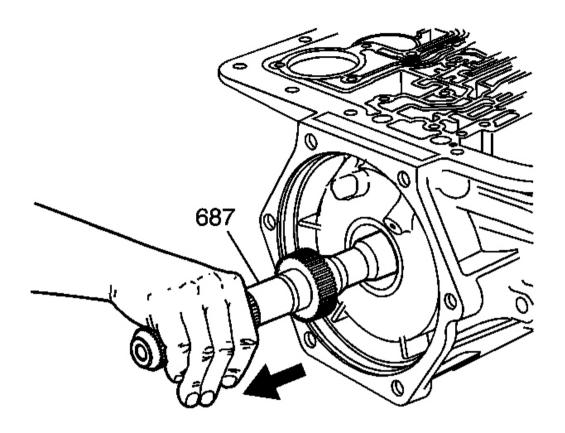
Fig. 74: Locating Output Shaft Courtesy of GENERAL MOTORS CORP.
