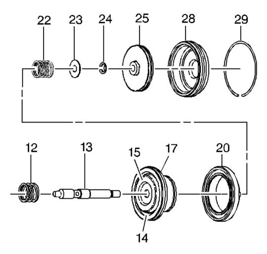
Fig. 305: Illustrating Assembly Order Of 2-4 servo components Courtesy of GENERAL MOTORS CORP.
