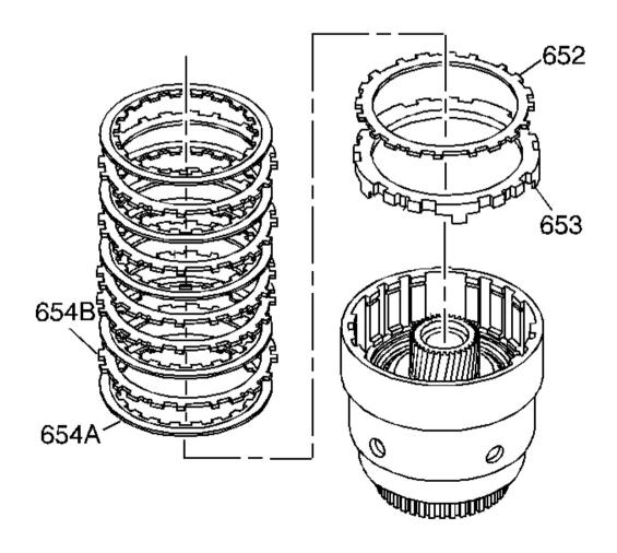
Fig. 181: Illustrating Clutch Plate Assembly
