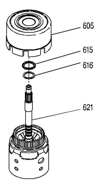
Fig. 145: View Of Stator Shaft/Selective Washer Bearing Assembly Courtesy of GENERAL MOTORS CORP.
