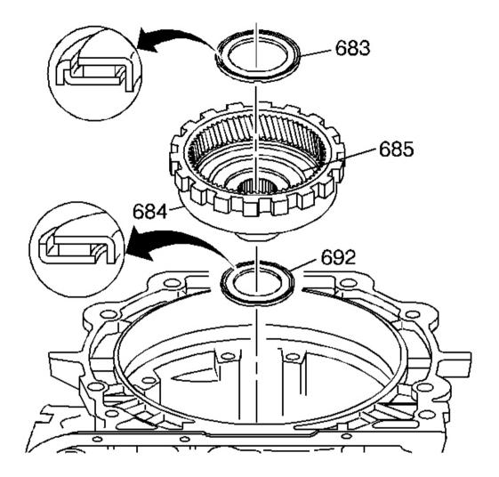
Fig. 109: View Of Reaction Carrier/Support Thrust Bearing Assembly Courtesy of GENERAL MOTORS CORP.
