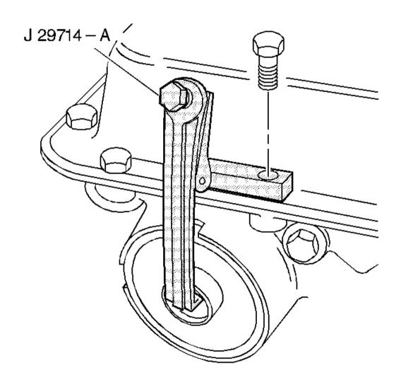
Fig. 26: Installing J 29714-A Courtesy of GENERAL MOTORS CORP.
