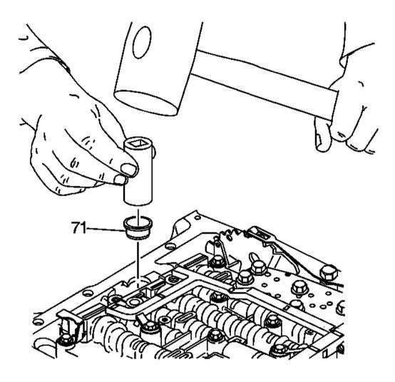
Fig. 296: Locating Oil Filter Seal Courtesy of GENERAL MOTORS CORP.
