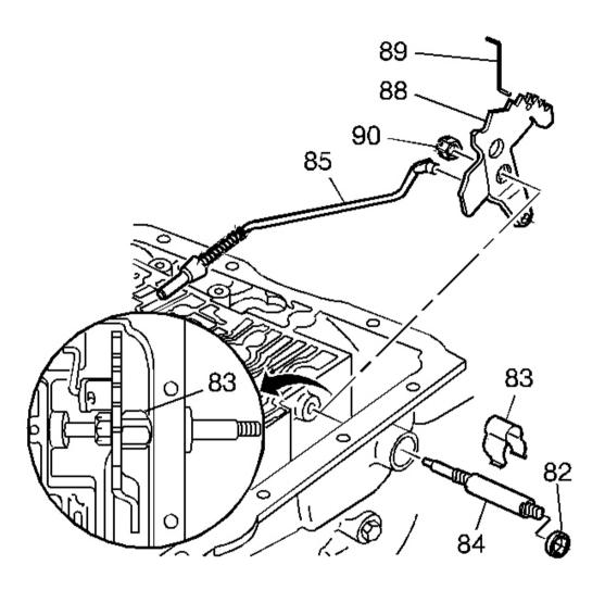
Fig. 104: Identifying Inner Manual Linkage Inspection Areas Courtesy of GENERAL MOTORS CORP.
