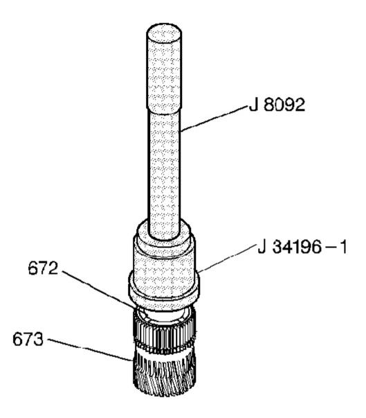
Fig. 124: Installing Reaction Sun Bushing Courtesy of GENERAL MOTORS CORP.
