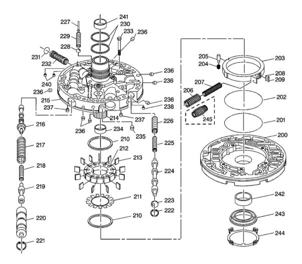
Fig. 5: Oil Pump Assembly Disassembled View Courtesy of GENERAL MOTORS CORP.
