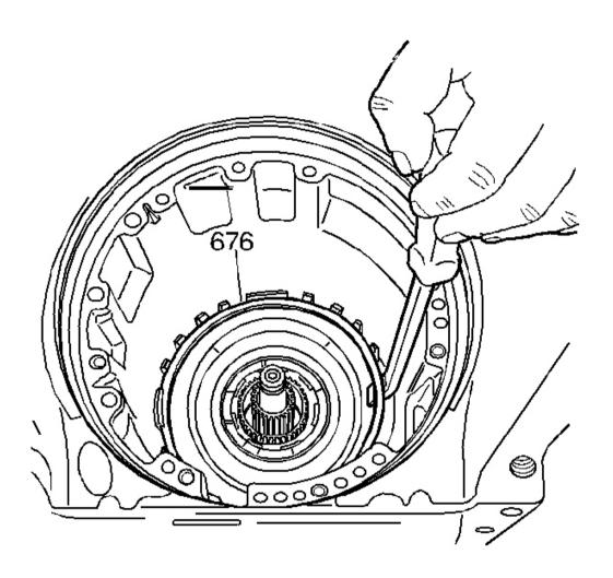
Fig. 121: Identifying Low And Reverse Support Retainer Ring Courtesy of GENERAL MOTORS CORP.
