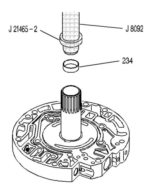
Fig. 230: View Of Stator Shaft Front Bushing Courtesy of GENERAL MOTORS CORP.
