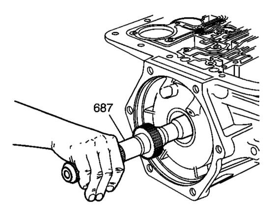
Fig. 136: View Of Output Shaft Courtesy of GENERAL MOTORS CORP.
