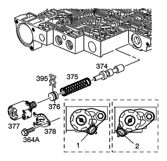
Fig. 266: Locating Actuator Feed Limit Valve & Pressure Control Solenoid Courtesy of GENERAL MOTORS CORP.
