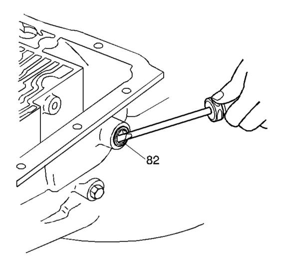
Fig. 80: Removing Manual Shaft Seal Courtesy of GENERAL MOTORS CORP.
