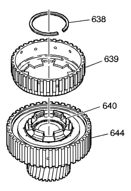
Fig. 174: Locating Overrun Clutch Hub Courtesy of GENERAL MOTORS CORP.
