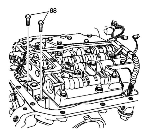
Fig. 43: Identifying TCC Solenoid Valve Mounting Bolts Courtesy of GENERAL MOTORS CORP.
