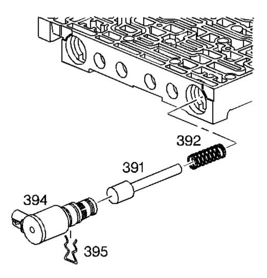
Fig. 255: Identifying 3-2 Control Valve & 3-2 Control Solenoid Courtesy of GENERAL MOTORS CORP.
