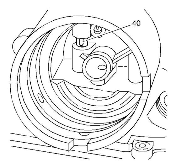
Fig. 96: Aligning Third Accumulator Retainer And Ball Assembly With Retainer Slot Courtesy of GENERAL MOTORS CORP.
