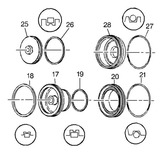
Fig. 303: 2-4 Servo Assembly Components Courtesy of GENERAL MOTORS CORP.
