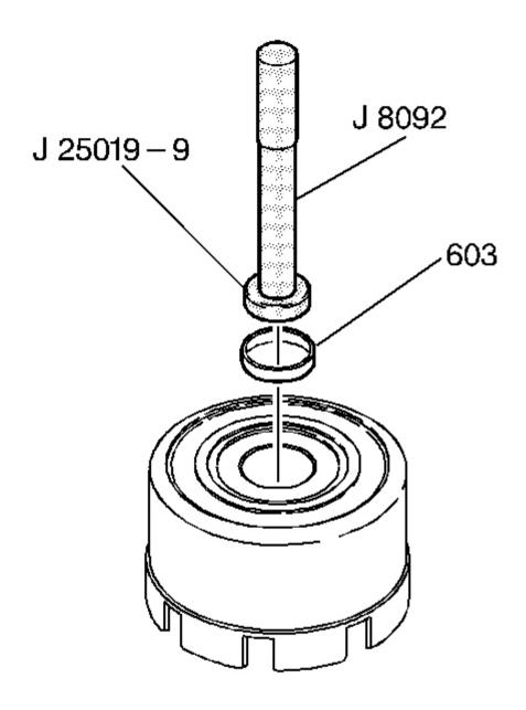
Fig. 193: View Of Reverse Input Clutch Front Bushing Courtesy of GENERAL MOTORS CORP.
