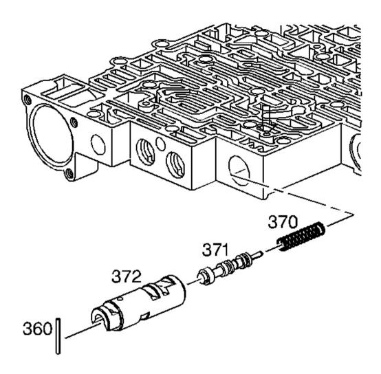
Fig. 253: View Of 1-2 Accumulator Valve & 1-2 Accumulator Valve Sleeve Courtesy of GENERAL MOTORS CORP.
