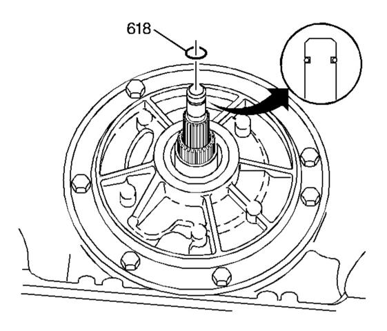
Fig. 248: Identifying Turbine Shaft O-Ring Courtesy of GENERAL MOTORS CORP.
