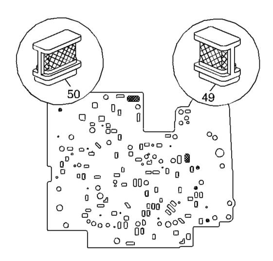
Fig. 278: Identifying Solenoid Screens Courtesy of GENERAL MOTORS CORP.
