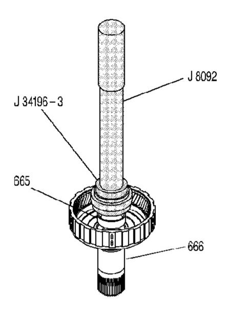
Fig. 130: Installing Reaction Carrier Shaft Front Bushing Courtesy of GENERAL MOTORS CORP.
