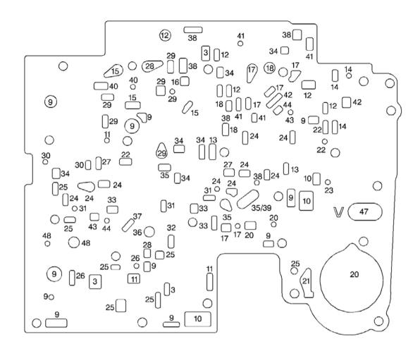
Fig. 342: Spacer Plate to Control Valve Body Gasket Courtesy of GENERAL MOTORS CORP.
