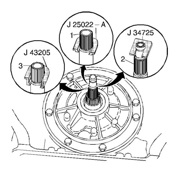
Fig. 243: Identifying Different End Play Fixture Adapters Courtesy of GENERAL MOTORS CORP.
