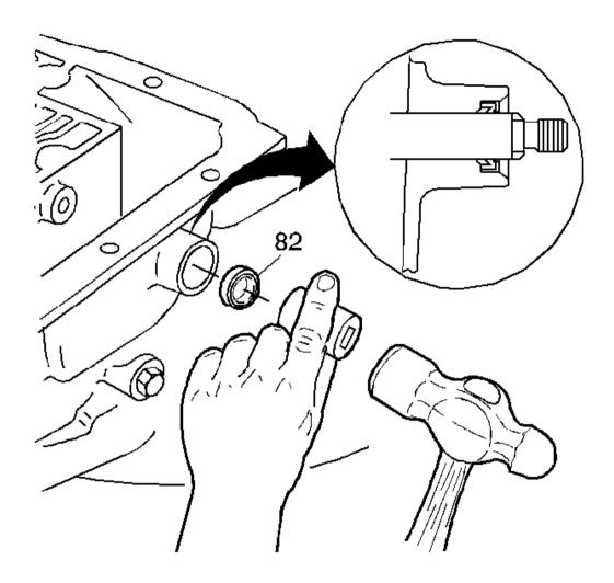
Fig. 99: Installing Manual Shaft Seal Courtesy of GENERAL MOTORS CORP.
