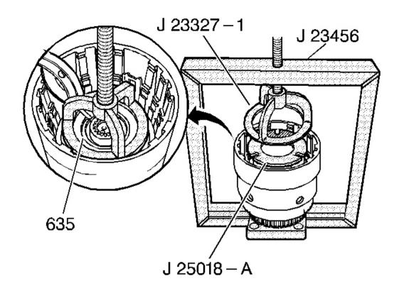
Fig. 164: Locating Overrun Clutch Spring Retainer Snap Ring Courtesy of GENERAL MOTORS CORP.
