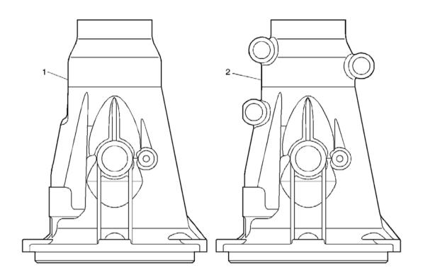
Fig. 21: Case Extension Identification Courtesy of GENERAL MOTORS CORP.
