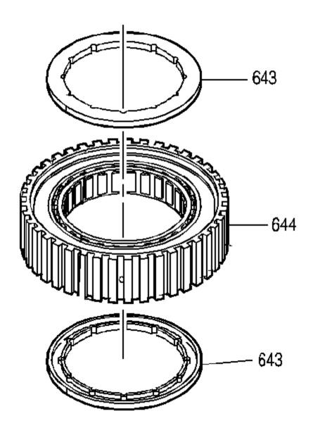
Fig. 172: View Of Sprag Assembly Retainer Rings Courtesy of GENERAL MOTORS CORP.
