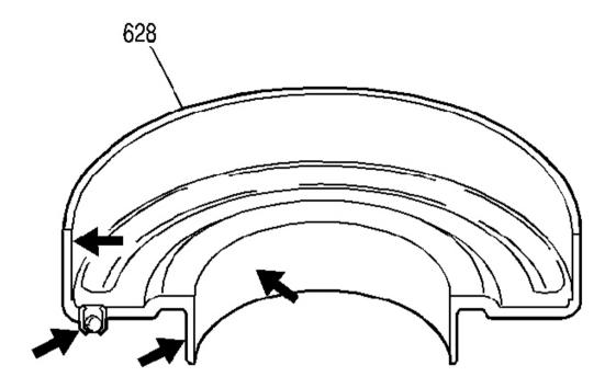
Fig. 155: Forward Clutch Housing Inspection Areas Courtesy of GENERAL MOTORS CORP.
