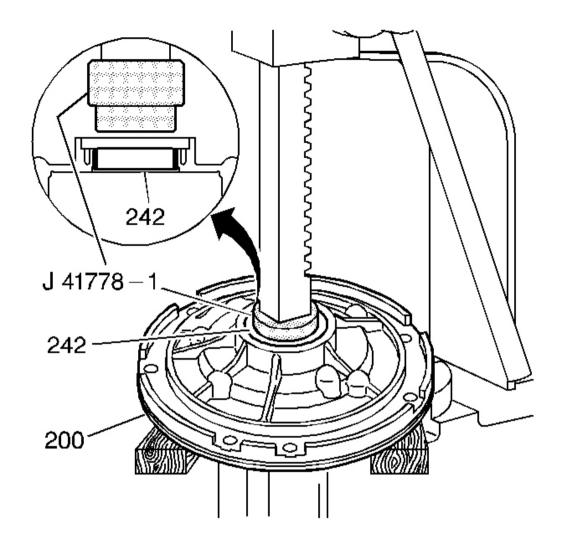
Fig. 214: Removing Pump Body Bushing Courtesy of GENERAL MOTORS CORP.
