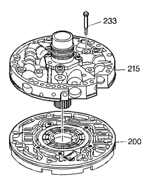
Fig. 207: Locating Pump Cover Bolts
