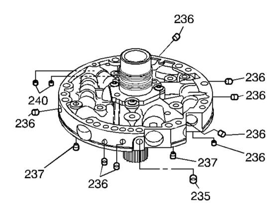
Fig. 226: Identifying Pump Cover Components Courtesy of GENERAL MOTORS CORP.
