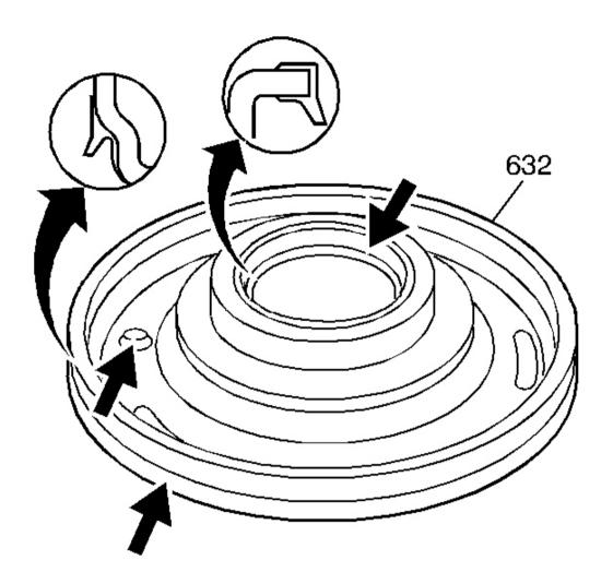
Fig. 160: Inspection Areas On Overrun Clutch Piston Courtesy of GENERAL MOTORS CORP.
