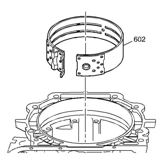
Fig. 204: View Of 2-4 Band Assembly Courtesy of GENERAL MOTORS CORP.
