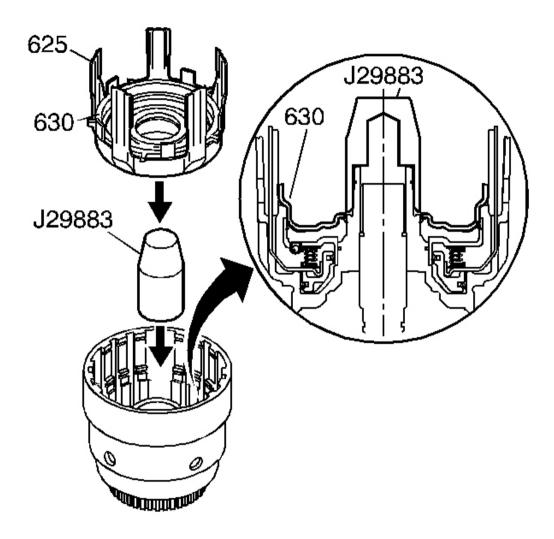
Fig. 159: View Of J 29883 Installed In Input Housing Courtesy of GENERAL MOTORS CORP.
