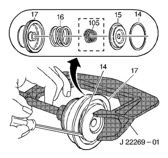
Fig. 300: Locating Servo Cushion Outer & Inner Spring With Retainer Courtesy of GENERAL MOTORS CORP.
