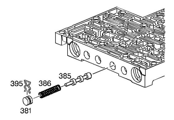
Fig. 257: Locating 3-4 Shift Valve Courtesy of GENERAL MOTORS CORP.
