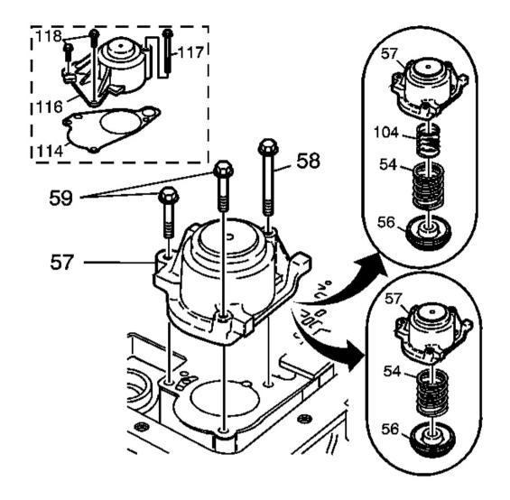
Fig. 50: Views Of 1-2 Accumulator Assemblies Courtesy of GENERAL MOTORS CORP.
