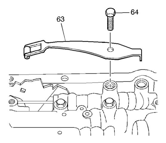
Fig. 293: View Of Manual Detent Spring Assembly Courtesy of GENERAL MOTORS CORP.
