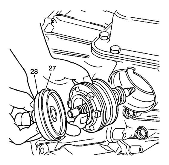
Fig. 306: View Of 2-4 Servo Assembly Courtesy of GENERAL MOTORS CORP.
