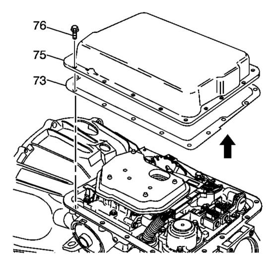
Fig. 299: View Of Transmission Oil Pan & Gasket Courtesy of GENERAL MOTORS CORP.
