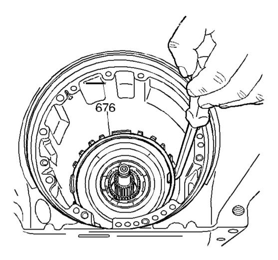
Fig. 71: Removing Low And Reverse Support Retainer Ring Courtesy of GENERAL MOTORS CORP.
