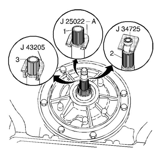
Fig. 56: Identifying Different End Play Fixture Adapters Courtesy of GENERAL MOTORS CORP.
