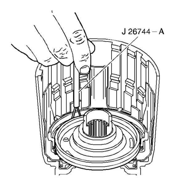
Fig. 162: Installing Overrun Clutch Piston Outer Seal With J 26744-A Courtesy of GENERAL MOTORS CORP.
