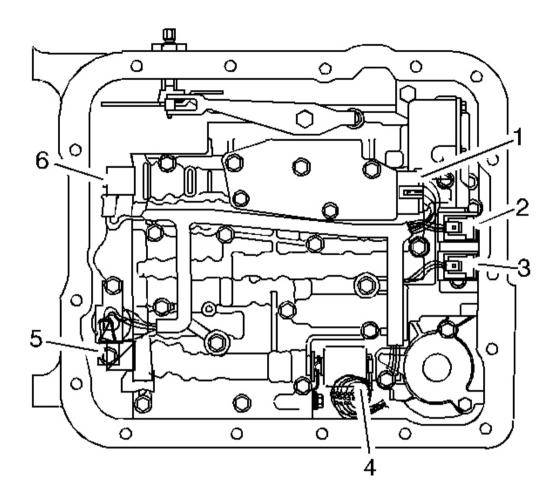
Fig. 41: Identifying Valve Body Electrical Connections Courtesy of GENERAL MOTORS CORP.
