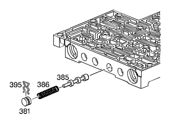
Fig. 263: Locating 3-4 Shift Valve Courtesy of GENERAL MOTORS CORP.
