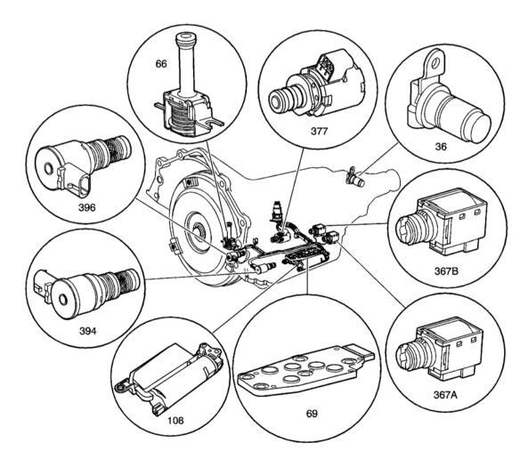
Fig. 11: Electronic Component View
