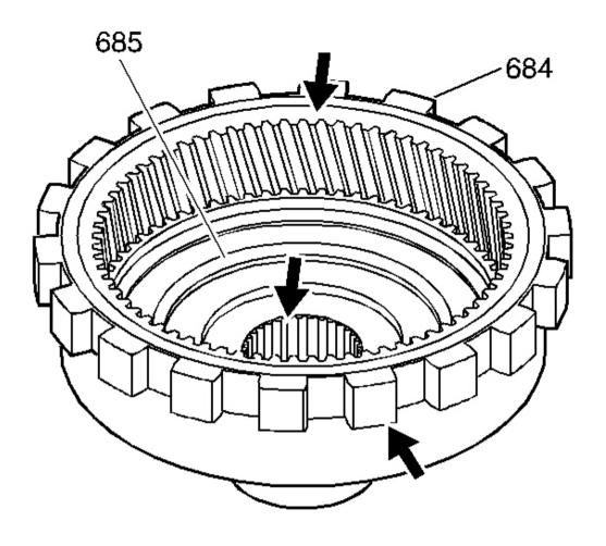
Fig. 106: View Of Reaction Gear And Carrier Inspection Areas Courtesy of GENERAL MOTORS CORP.
