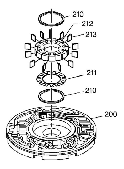
Fig. 221: Identifying Pump Vane Ring Assemblies Courtesy of GENERAL MOTORS CORP.
