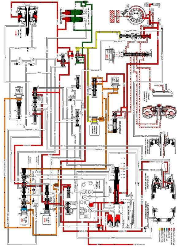
Fig. 327: Overdrive Range, Second Gear Courtesy of GENERAL MOTORS CORP.
