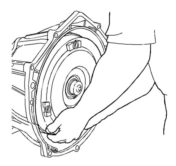
Fig. 23: Removing Torque Converter Courtesy of GENERAL MOTORS CORP.
