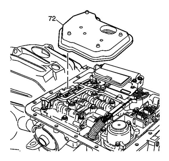
Fig. 297: View Of Transmission Oil Filter Assembly Courtesy of GENERAL MOTORS CORP.
