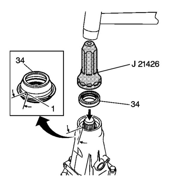
Fig. 318: Locating Case Extension Oil Seal Assembly Courtesy of GENERAL MOTORS CORP.
