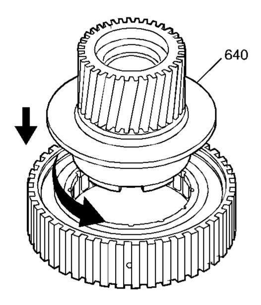
Fig. 173: Inspection Areas On Forward Sprag Clutch Inner Race And Input Sun Gear Assembly Courtesy of GENERAL MOTORS CORP.
