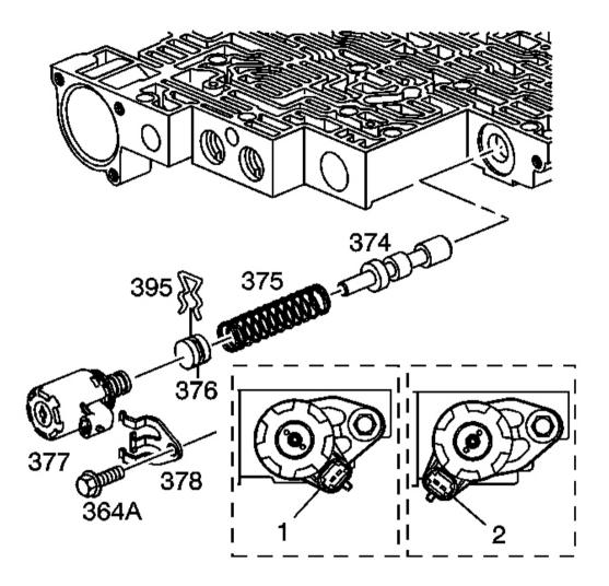
Fig. 254: Locating Actuator Feed Limit Valve & Pressure Control Solenoid Courtesy of GENERAL MOTORS CORP.
