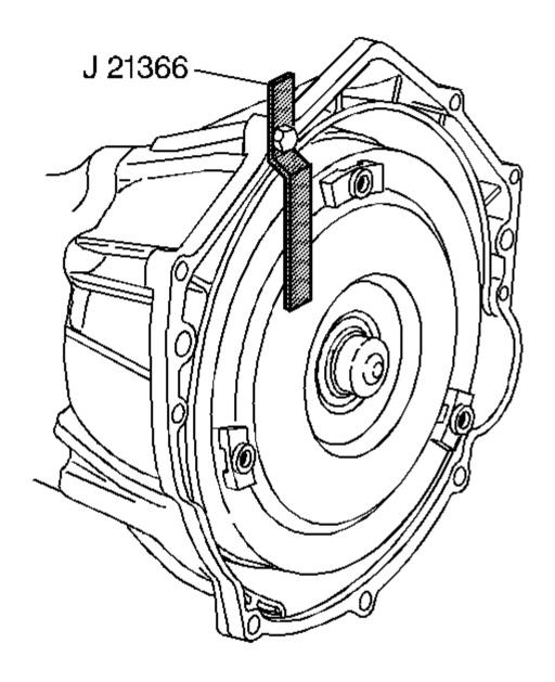
Fig. 320: View Of J 21366 Installed On Torque Converter Courtesy of GENERAL MOTORS CORP.
