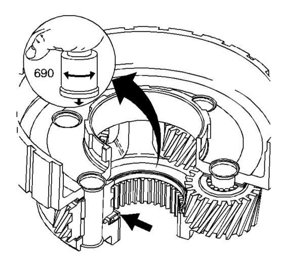
Fig. 108: Illustrating Proper Inspection Of Reaction Carrier Captive Thrust Bearing Courtesy of GENERAL MOTORS CORP.
