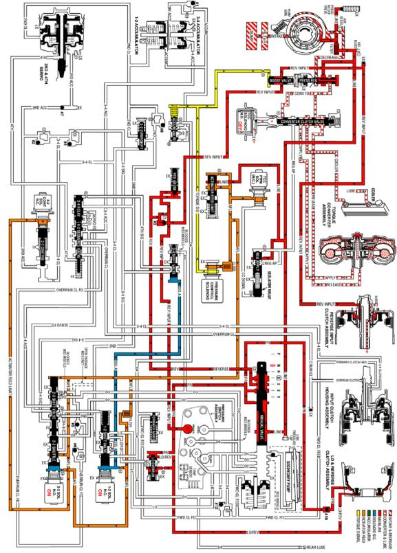
Fig. 324: Reverse Courtesy of GENERAL MOTORS CORP.
