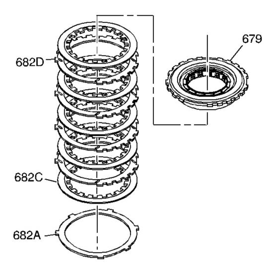
Fig. 112: View Of Low And Reverse Clutch Plate Assembly Courtesy of GENERAL MOTORS CORP.
