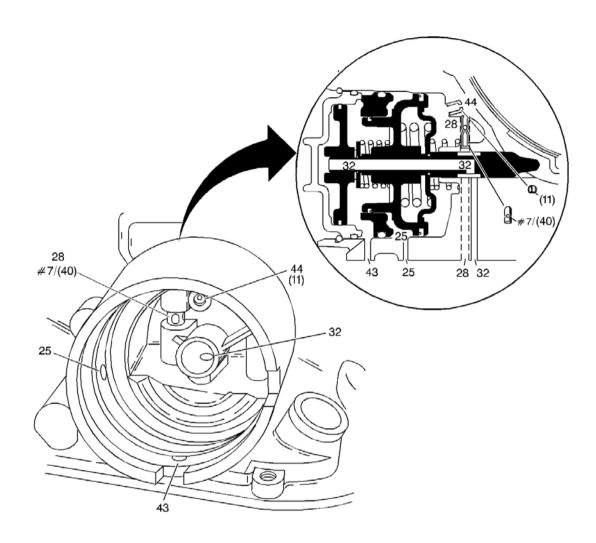
Fig. 344: 2-4 Servo Fluid Passages
