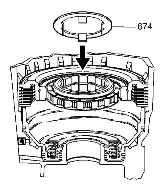
Fig. 126: Aligning Thrust Washer Tangs With Low And Reverse Roller Clutch Race Splines Courtesy of GENERAL MOTORS CORP.
