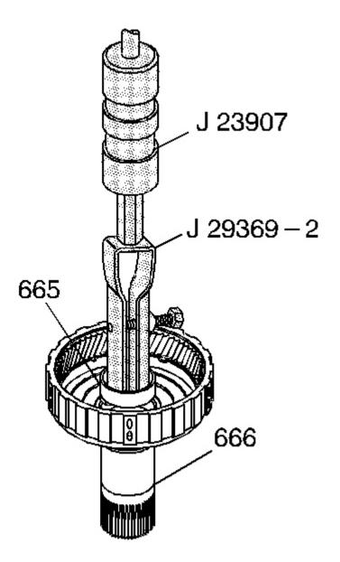
Fig. 128: Removing Reaction Carrier Shaft Front Bushing Courtesy of GENERAL MOTORS CORP.
