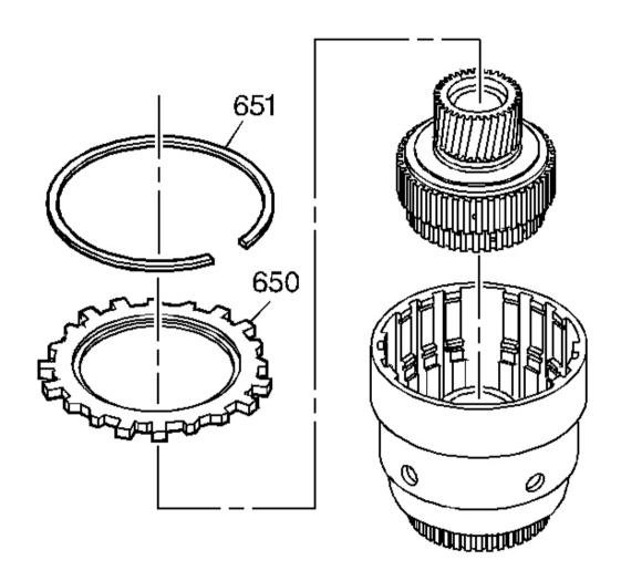
Fig. 147: Identifying Forward Clutch Selective Backing Plate & Retainer Ring Courtesy of GENERAL MOTORS CORP.
