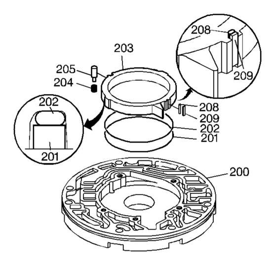
Fig. 219: Identifying Pump Slide Components Courtesy of GENERAL MOTORS CORP.
