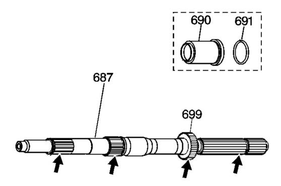
Fig. 133: Identifying Output Shaft Seal & Output Shaft Sleeve Courtesy of GENERAL MOTORS CORP.
