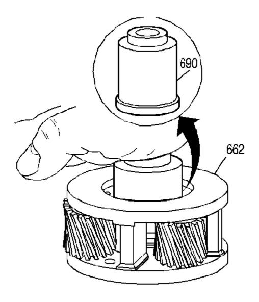
Fig. 141: View Of Input Carrier Captive Thrust Bearing Assembly Courtesy of GENERAL MOTORS CORP.
