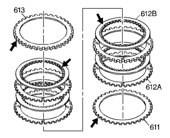
Fig. 199: Inspecting Plates For Damage Or Wear Courtesy of GENERAL MOTORS CORP.
