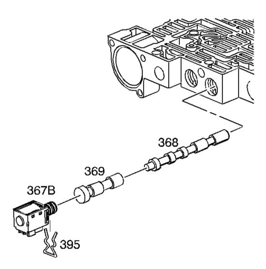
Fig. 268: Identifying 2-3 Shuttle Valve & Solenoid Components Courtesy of GENERAL MOTORS CORP.
