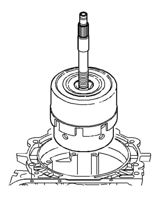
Fig. 203: Identifying Reverse Input & Input Clutch Assembly Courtesy of GENERAL MOTORS CORP.
