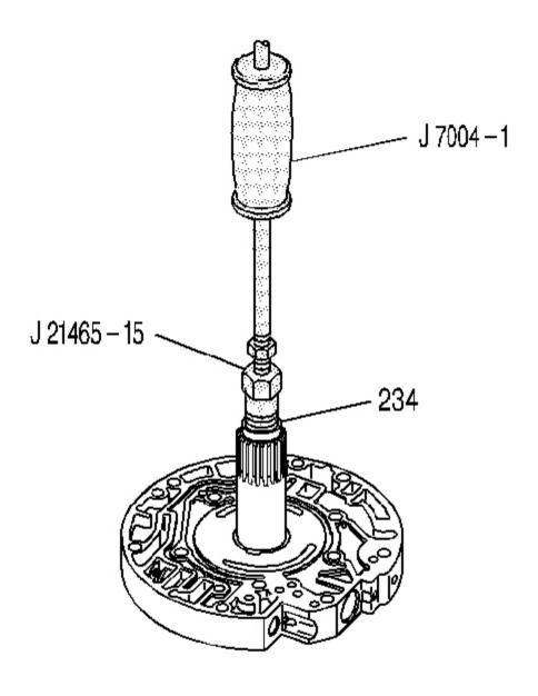
Fig. 228: Locating Stator Shaft Front Bushing Courtesy of GENERAL MOTORS CORP.
