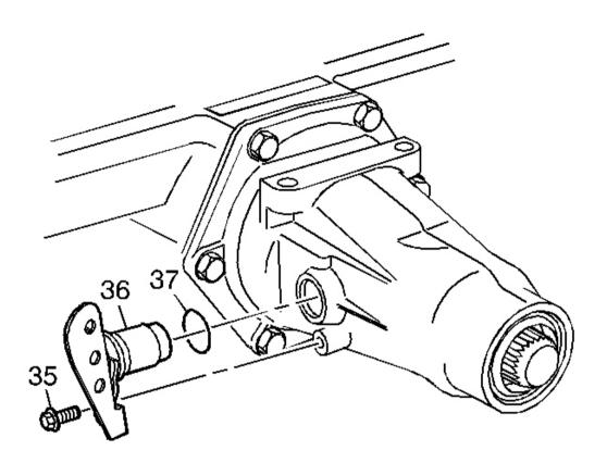
Fig. 317: View Of Internal Transmission Speed Sensor Courtesy of GENERAL MOTORS CORP.
