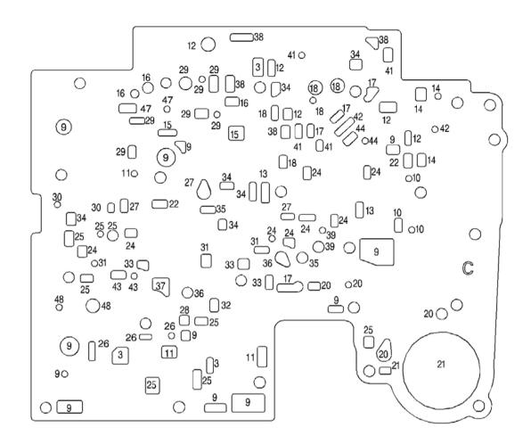
Fig. 340: Spacer Plate to Case Gasket - M30/M32 Courtesy of GENERAL MOTORS CORP.
