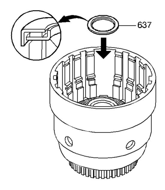
Fig. 168: Input Sun Gear Bearing Assembly Courtesy of GENERAL MOTORS CORP.
