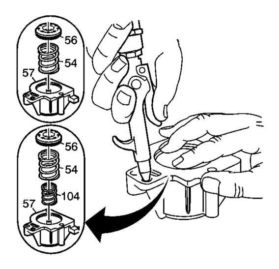
Fig. 274: View Of 1-2 Accumulator Components Courtesy of GENERAL MOTORS CORP.
