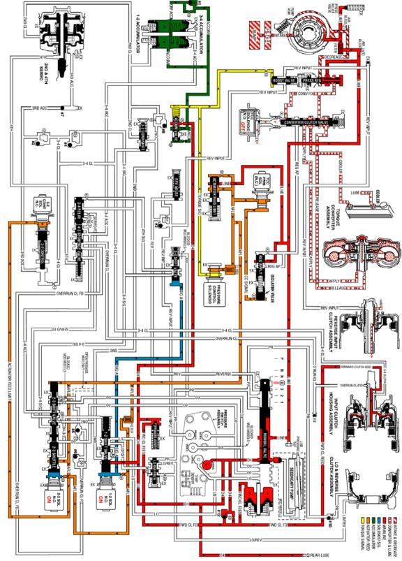
Fig. 326: Overdrive Range, First Gear Courtesy of GENERAL MOTORS CORP.
