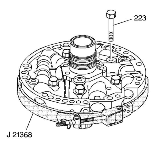
Fig. 236: Locating Pump Cover Bolts
