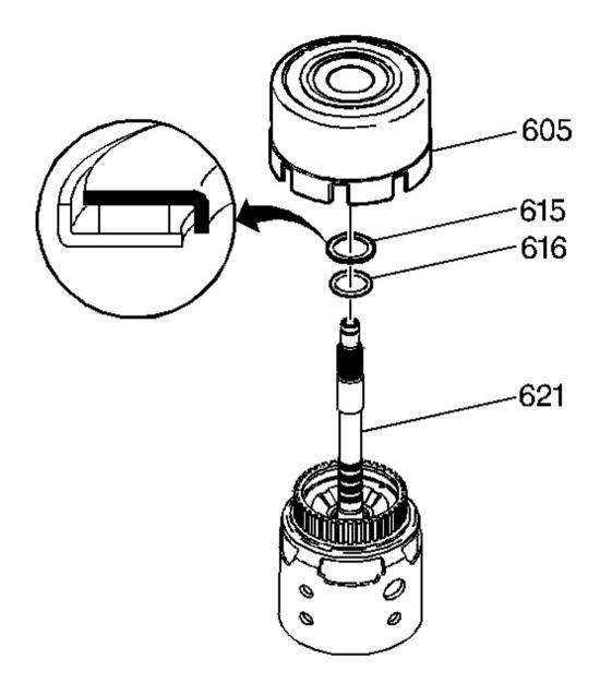
Fig. 202: Locating Selective Thrust Washer Courtesy of GENERAL MOTORS CORP.
