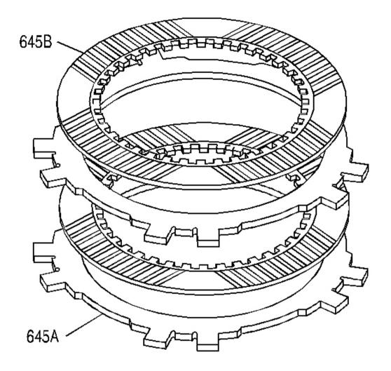
Fig. 166: Identifying Overrun Clutch Plates Courtesy of GENERAL MOTORS CORP.
