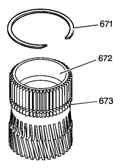
Fig. 122: Inspection Areas On Reaction Sun Gear Courtesy of GENERAL MOTORS CORP.
