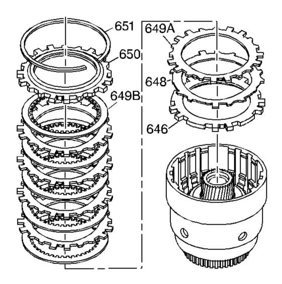
Fig. 177: Identifying Forward Clutch Apply Plates Courtesy of GENERAL MOTORS CORP.
