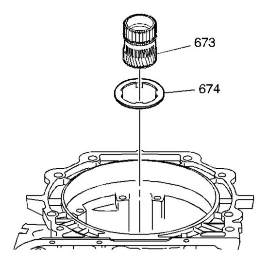
Fig. 70: Identifying Reaction Sun Gear & Thrust Washer Courtesy of GENERAL MOTORS CORP.
