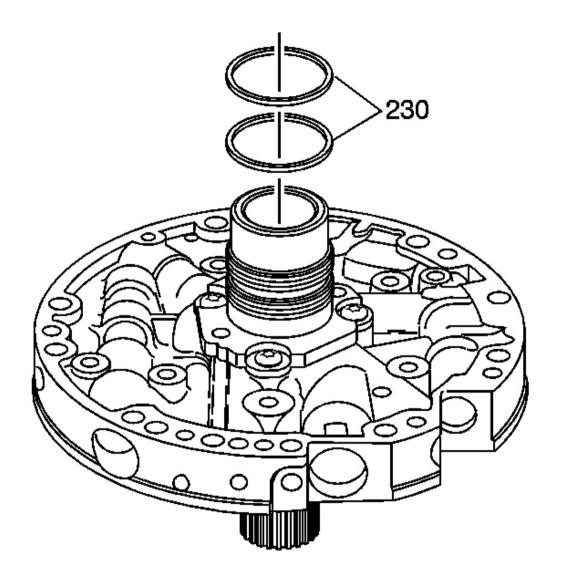
Fig. 225: Locating Stator Shaft Oil Seal Rings Courtesy of GENERAL MOTORS CORP.
