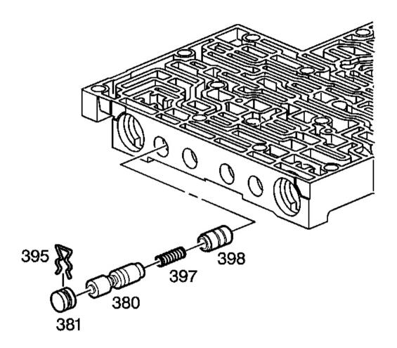
Fig. 258: Identifying Isolator Valve & Regulator Apply Valve Courtesy of GENERAL MOTORS CORP.
