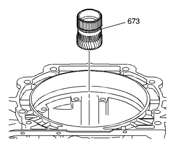
Fig. 125: Identifying Reaction Sun Gear Courtesy of GENERAL MOTORS CORP.
