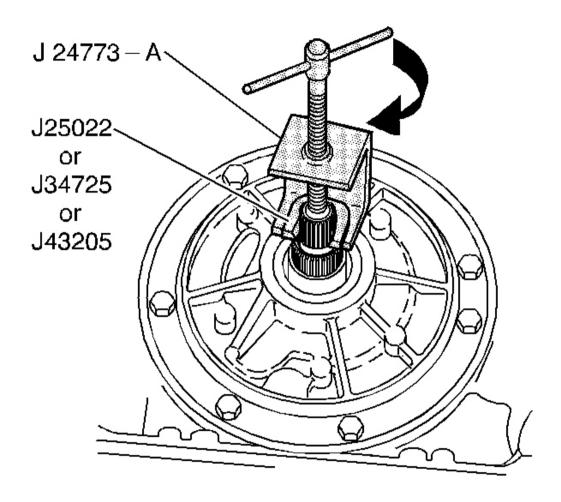
Fig. 244: Identifying J 24773-A Courtesy of GENERAL MOTORS CORP.
