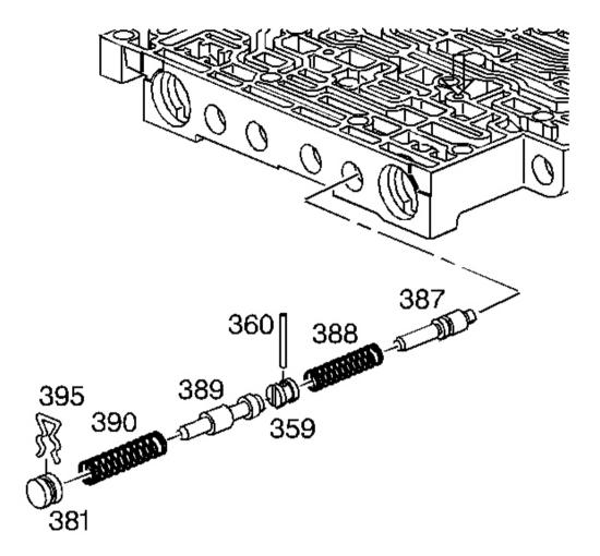
Fig. 256: View Of Reverse Abuse Valve & 3-2 Downshift Valve Courtesy of GENERAL MOTORS CORP.
