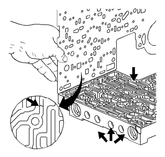
Fig. 260: Inspecting Control Valve Body For Channel Witness Marks Courtesy of GENERAL MOTORS CORP.
