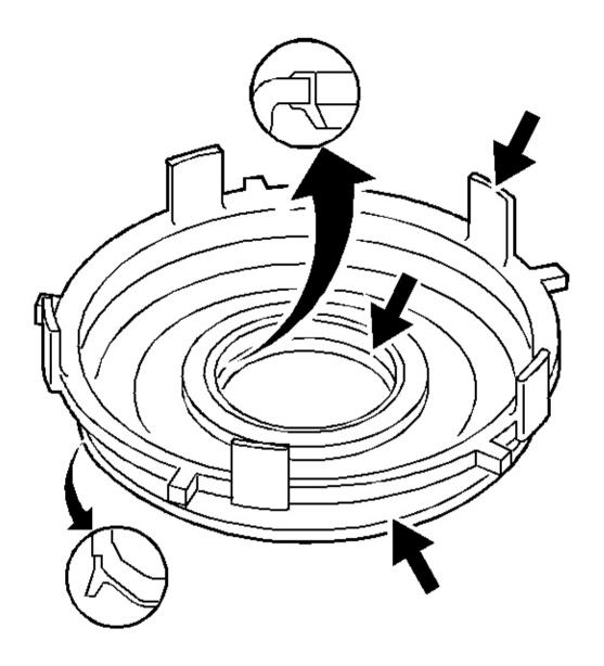
Fig. 156: Inspecting Forward Clutch Piston For Damage Or Wear Courtesy of GENERAL MOTORS CORP.
