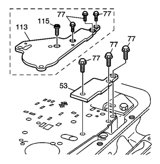
Fig. 51: View Of Spacer Plate Support Plate & Bolts Courtesy of GENERAL MOTORS CORP.
