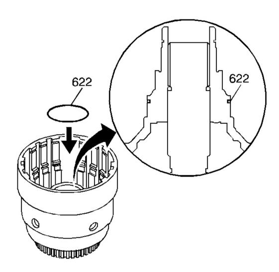
Fig. 153: Locating Forward Clutch Housing O-Ring Seal Courtesy of GENERAL MOTORS CORP.
