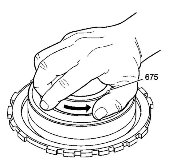
Fig. 118: Checking Low And Reverse Roller Clutch Race Rotation Courtesy of GENERAL MOTORS CORP.
