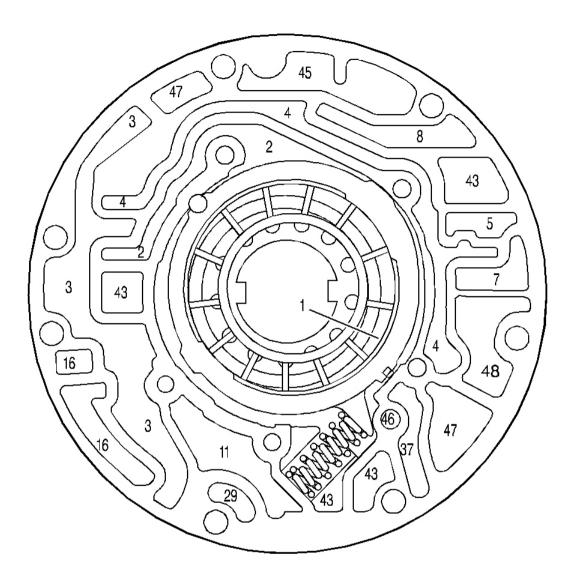
Fig. 335: Pump Body Fluid Passages (Pump Cover Side) Courtesy of GENERAL MOTORS CORP.
