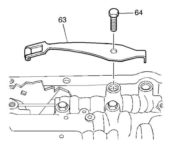
Fig. 46: View Of Manual Detent Spring Assembly Courtesy of GENERAL MOTORS CORP.
