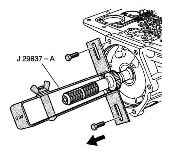
Fig. 144: Identifying J 29837-A Courtesy of GENERAL MOTORS CORP.
