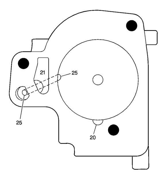
Fig. 345: 1-2 Accumulator Cover Fluid Passages Courtesy of GENERAL MOTORS CORP.
