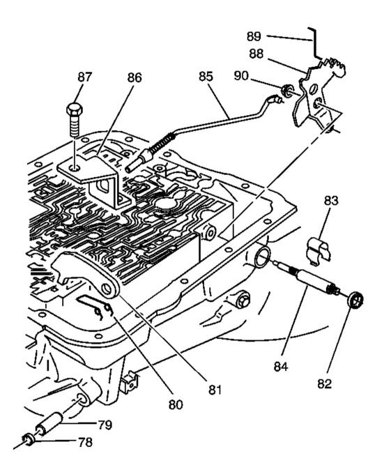
Fig. 10: Parking Lock & Manual Shift Shaft Assembly Disassembled View Courtesy of GENERAL MOTORS CORP.
