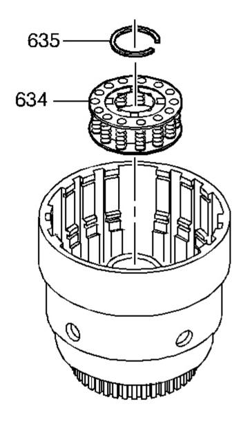
Fig. 163: View Of Overrun Clutch Spring Assembly Courtesy of GENERAL MOTORS CORP.
