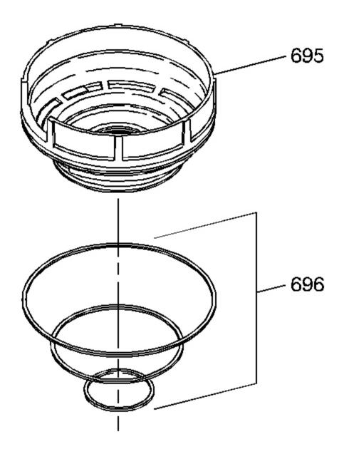
Fig. 100: Installing Transmission Seals Onto Low And Reverse Clutch Piston Courtesy of GENERAL MOTORS CORP.
