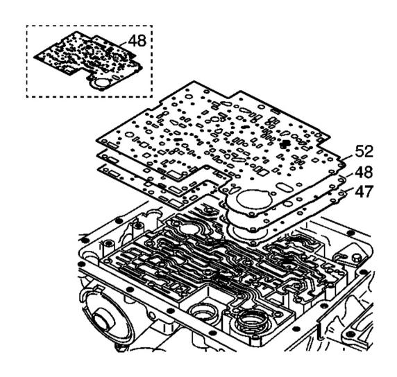
Fig. 52: Identifying Valve Body Gasket Courtesy of GENERAL MOTORS CORP.
