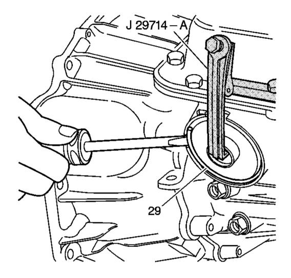
Fig. 309: Locating Servo Cover Retaining Ring Courtesy of GENERAL MOTORS CORP.
