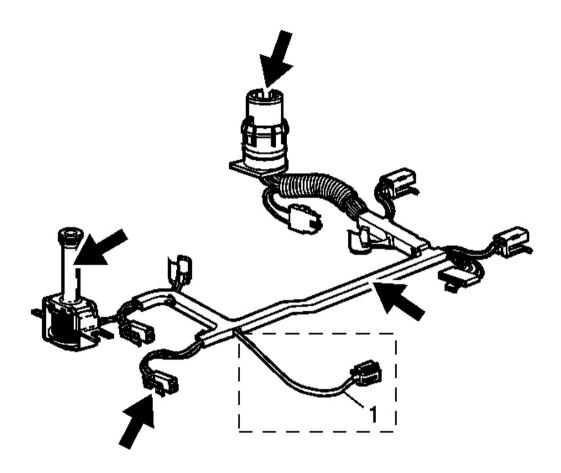
Fig. 283: Locating Wiring Harness And Solenoid Assembly Inspection Areas Courtesy of GENERAL MOTORS CORP.
