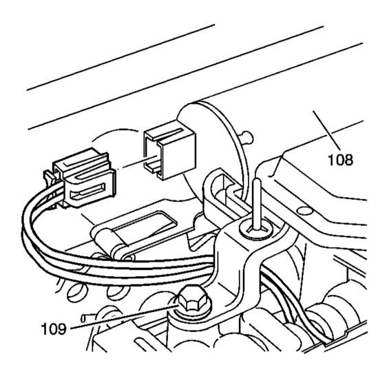
Fig. 295: View Of Wiring Harness Connector For Secondary Fluid Pump Courtesy of GENERAL MOTORS CORP.
