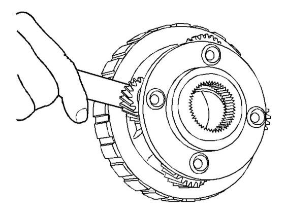
Fig. 107: Checking Reaction Carrier Pinion End Play With Feeler Gage Courtesy of GENERAL MOTORS CORP.
