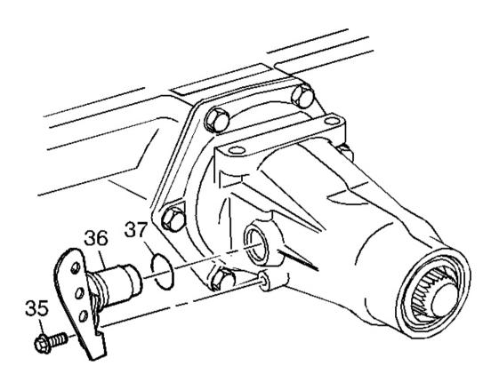
Fig. 33: View Of Internal Transmission Speed Sensor Courtesy of GENERAL MOTORS CORP.
