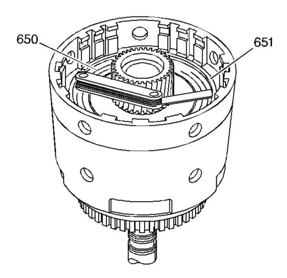
Fig. 178: Measuring Forward Clutch Plate Travel Courtesy of GENERAL MOTORS CORP.
