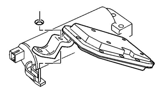
Fig. 298: View Of Secondary Fluid Pump & Clip Courtesy of GENERAL MOTORS CORP.
