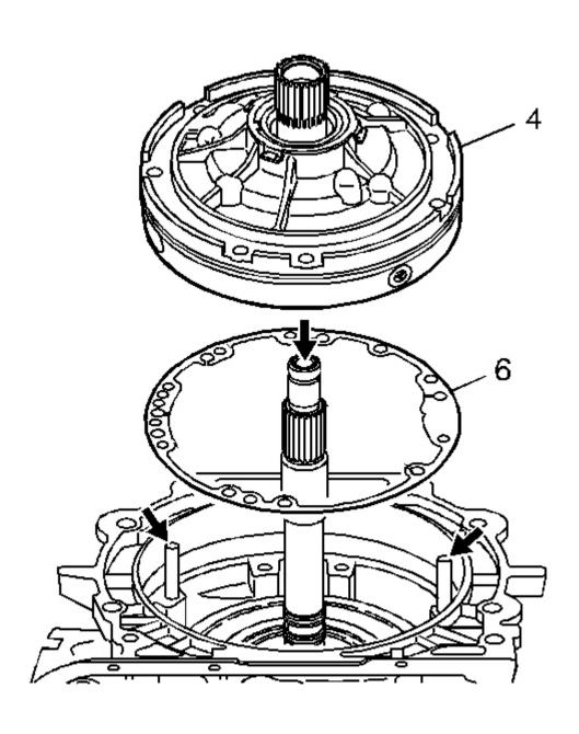
Fig. 240: Aligning Pump Cover To Case Gasket Courtesy of GENERAL MOTORS CORP.
