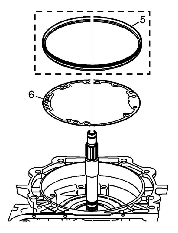
Fig. 62: Identifying External Fluid Pump Seal Courtesy of GENERAL MOTORS CORP.
