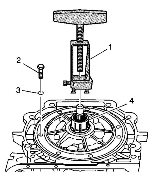
Fig. 60: Locating Pump Bolts Courtesy of GENERAL MOTORS CORP.
