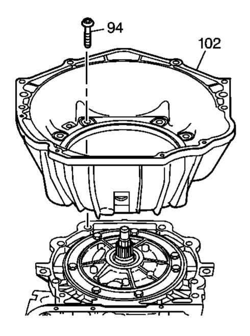
Fig. 25: View Of Converter Housing Bolts Courtesy of GENERAL MOTORS CORP.
