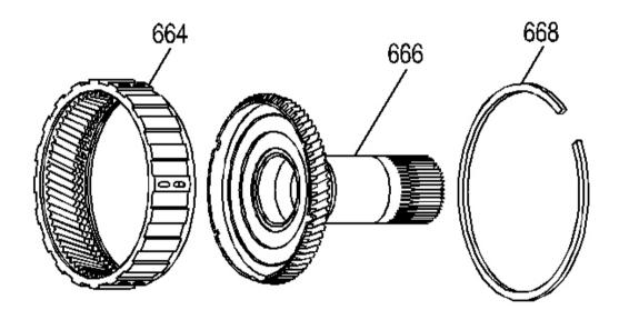
Fig. 127: Identifying Reaction Carrier Components Courtesy of GENERAL MOTORS CORP.
