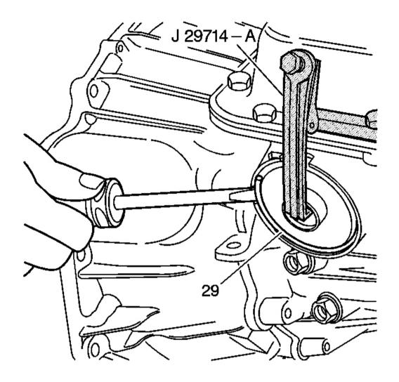
Fig. 28: Locating Servo Cover Retaining Ring Courtesy of GENERAL MOTORS CORP.
