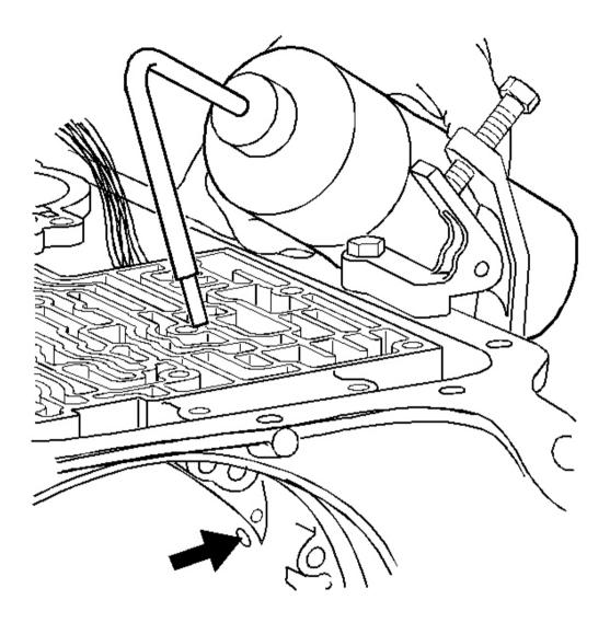
Fig. 91: Locating Small Hole In Accumulator Courtesy of GENERAL MOTORS CORP.
