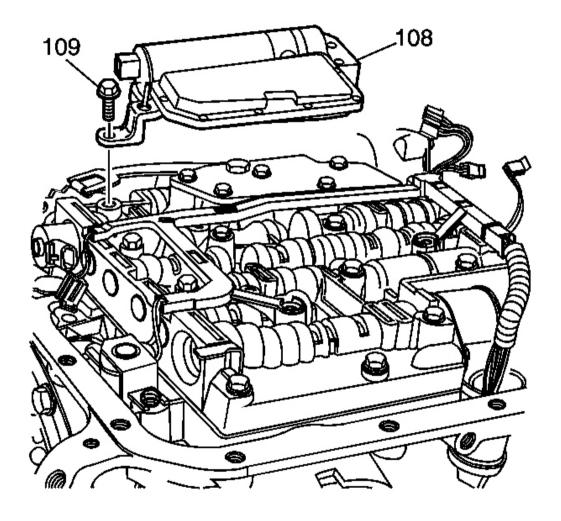
Fig. 294: Identifying Secondary Fluid Pump Courtesy of GENERAL MOTORS CORP.
