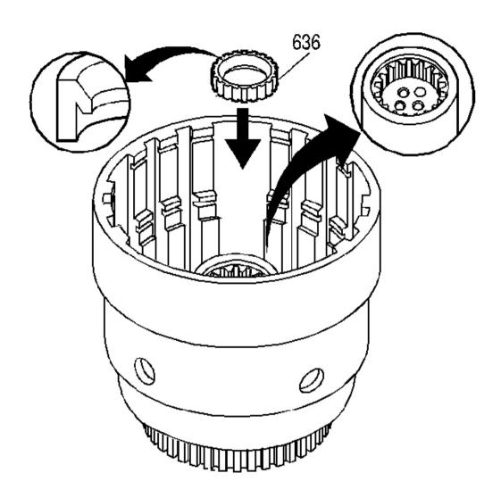
Fig. 165: View Of Input Housing To Output Shaft Seal Courtesy of GENERAL MOTORS CORP.
