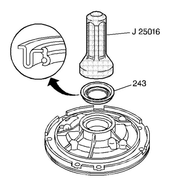
Fig. 217: Using J 25016 To Install Oil Seal Assembly Courtesy of GENERAL MOTORS CORP.
