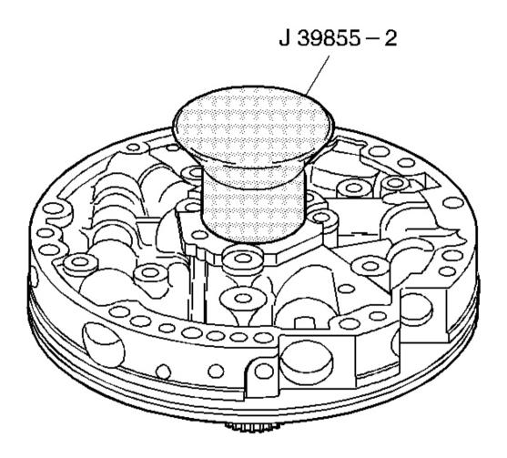
Fig. 238: Identifying J 39855-2 Courtesy of GENERAL MOTORS CORP.
