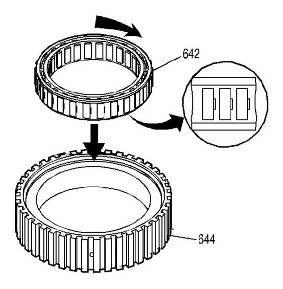
Fig. 171: Forward Sprag Assembly Courtesy of GENERAL MOTORS CORP.
