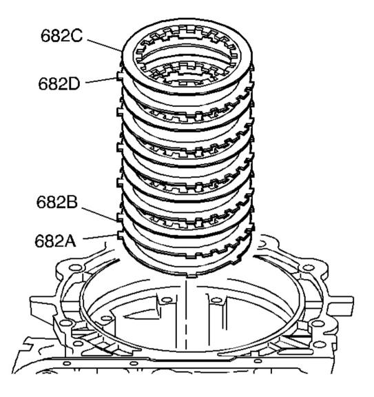
Fig. 77: Locating Low And Reverse Clutch Components Courtesy of GENERAL MOTORS CORP.
