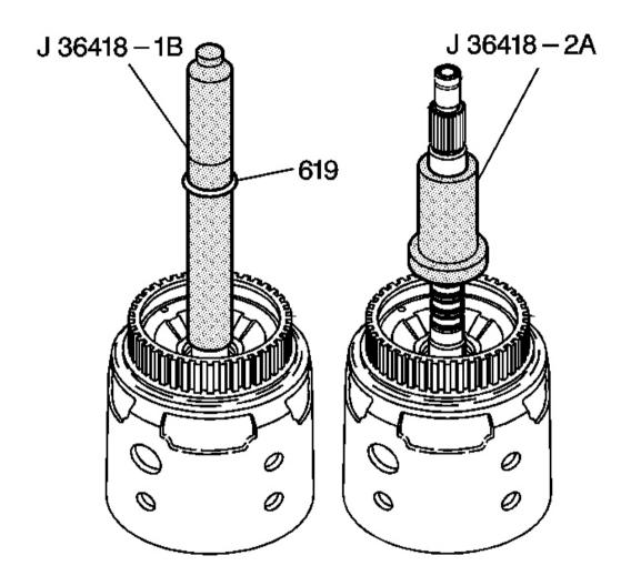
Fig. 186: Identifying J 36418-1B & J 36418-2A Courtesy of GENERAL MOTORS CORP.
