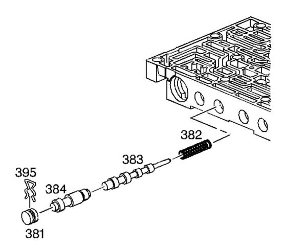
Fig. 259: View Of 4-3 Sequence Valve & 3-4 Relay Valve Courtesy of GENERAL MOTORS CORP.
