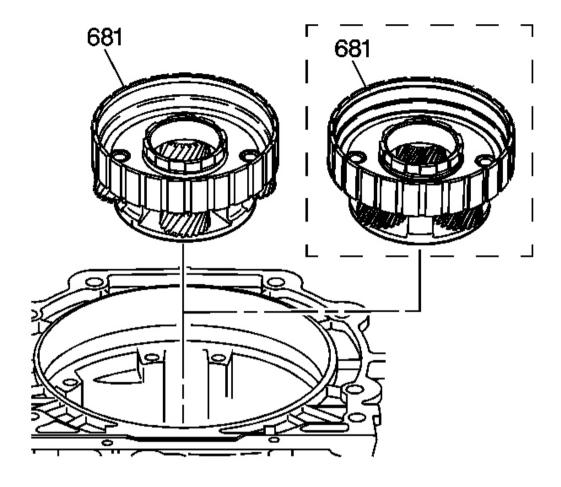
Fig. 110: Identifying Reaction Carrier Assembly Courtesy of GENERAL MOTORS CORP.
