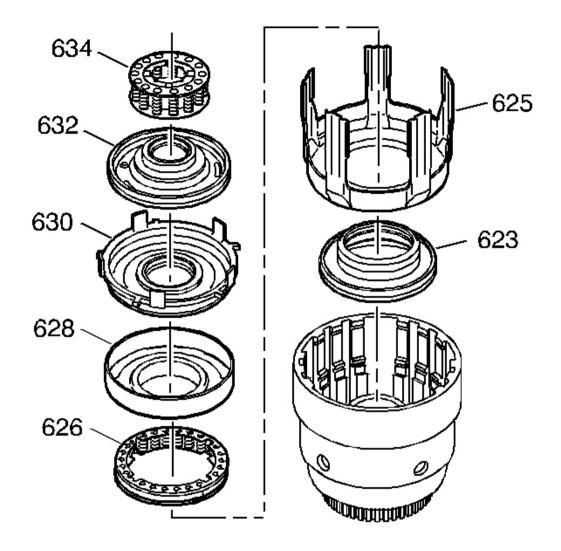
Fig. 150: Input Clutch Assembly Courtesy of GENERAL MOTORS CORP.
