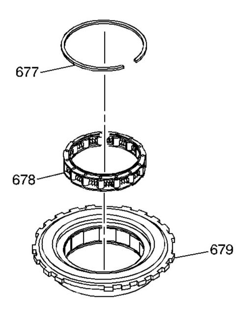
Fig. 117: Identifying Low And Reverse Roller Clutch Assembly Courtesy of GENERAL MOTORS CORP.
